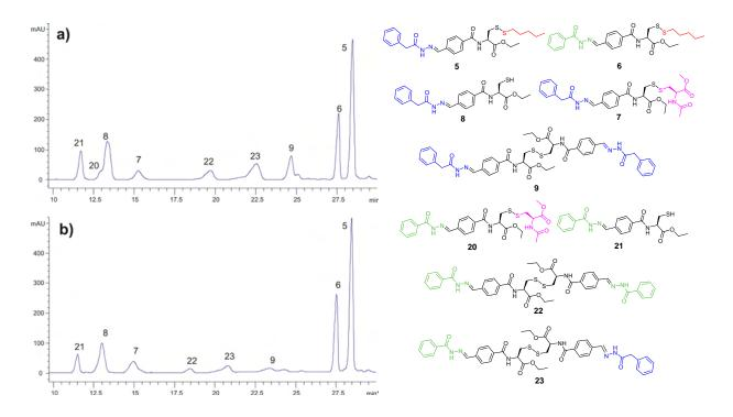
HPLC peaks were assigned by preparation of the individual components of the mixture. The presence of the expected compounds in the mixture was confirmed by ESI-MS using a Varian 1200 instrument (positive mode).
