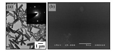
S3: SEM images of  $C_{60}$ : $C_{12}$ -xPPP 1:1 blend in toluene (a) spincoated at 100 rpm, (b) spincoated at 200 rpm, (c) spincoated at 500 rpm and (d) spincoated at 1000 rpm
