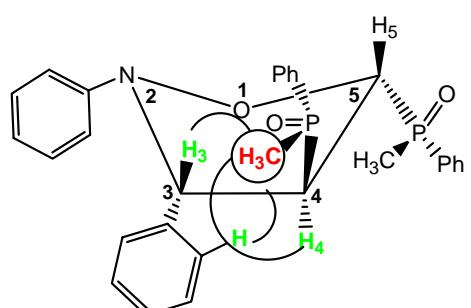
**Fig. 1** Irradiation (NOE) of CH<sub>3</sub> at  $\delta$  = 1.62 ppm
