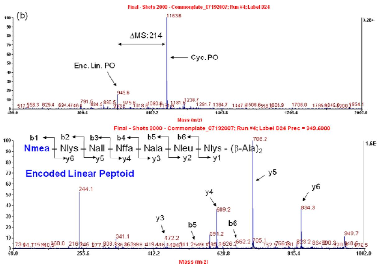
**Figure S5.** Sequence analysis for random members from cyclic peptoids library with Nmea at N-terminal: (b) Nmea-Nlys-Nall-Nffa-Nala-Nleu-Nlys.
