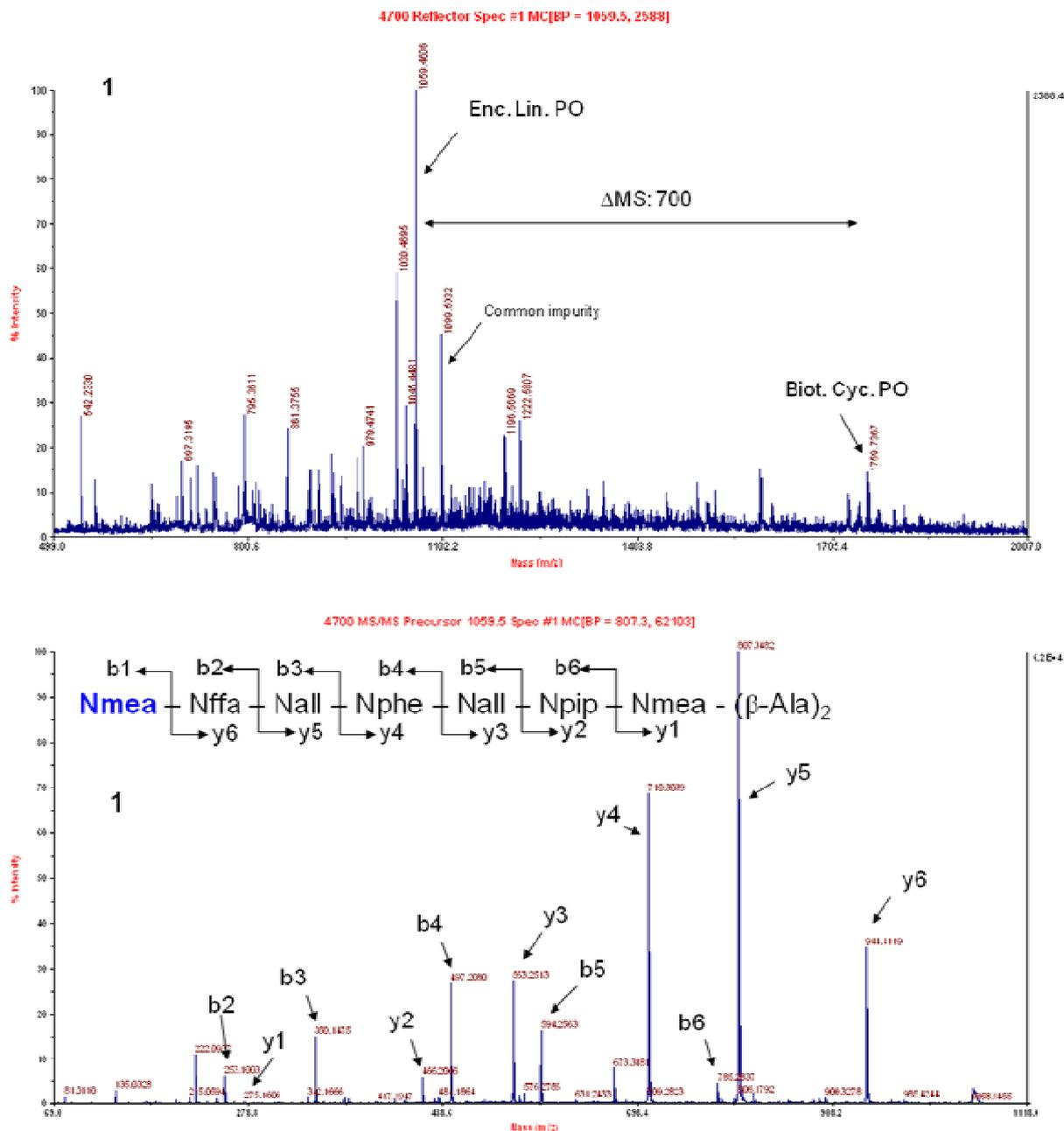
**Figure S8.** MS, MS/MS data for biotin-labeled cyclic peptide (**1**) with Nmea at N-terminal.
