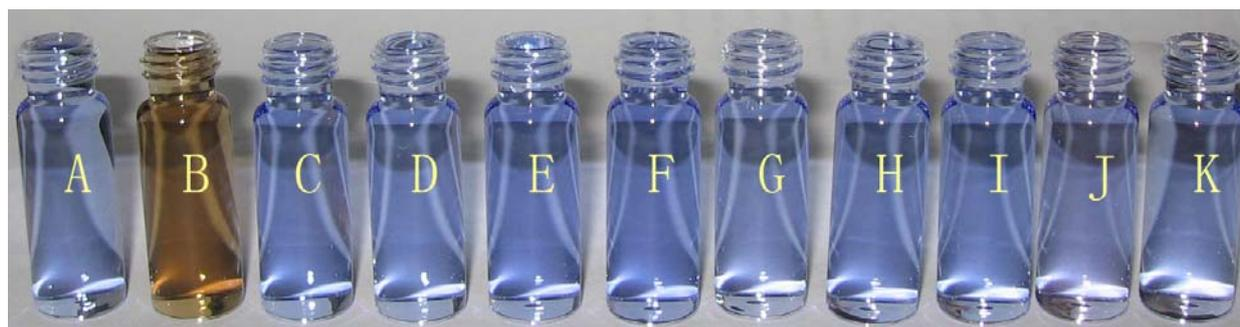
**Figure S9.** Different solutions of zincon and copper ions in water ( $5.0 \times 10^{-5}$  and  $2.2 \times 10^{-5}$  mol/L, respectively) in the presence of anion ( $5.0 \times 10^{-5}$  mol/L). From left to right: no anion,  $\text{CN}^-$ ,  $\text{Cl}^-$ ,  $\text{I}^-$ ,  $\text{IO}_3^-$ ,  $\text{SO}_4^{2-}$ ,  $\text{NO}_2^-$ ,  $\text{Br}^-$ ,  $\text{H}_2\text{PO}_4^-$ ,  $\text{HSO}_4^-$ ,  $\text{ClO}_4^-$ .
