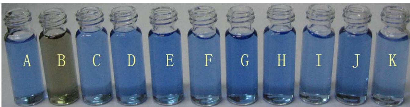
**Figure S11.** Different solutions of zincon and copper ions in water ( $5.0 \times 10^{-5}$  and  $2.2 \times 10^{-5}$  mol/L, respectively) in the presence of anion ( $5.0 \times 10^{-5}$  mol/L). From left to right: no anion,  $F^-$ ,  $Cl^-$ ,  $I^-$ ,  $IO_3^-$ ,  $SO_4^{2-}$ ,  $NO_2^-$ ,  $Br^-$ ,  $H_2PO_4^-$ ,  $HSO_4^-$ ,  $ClO_4^-$ .
