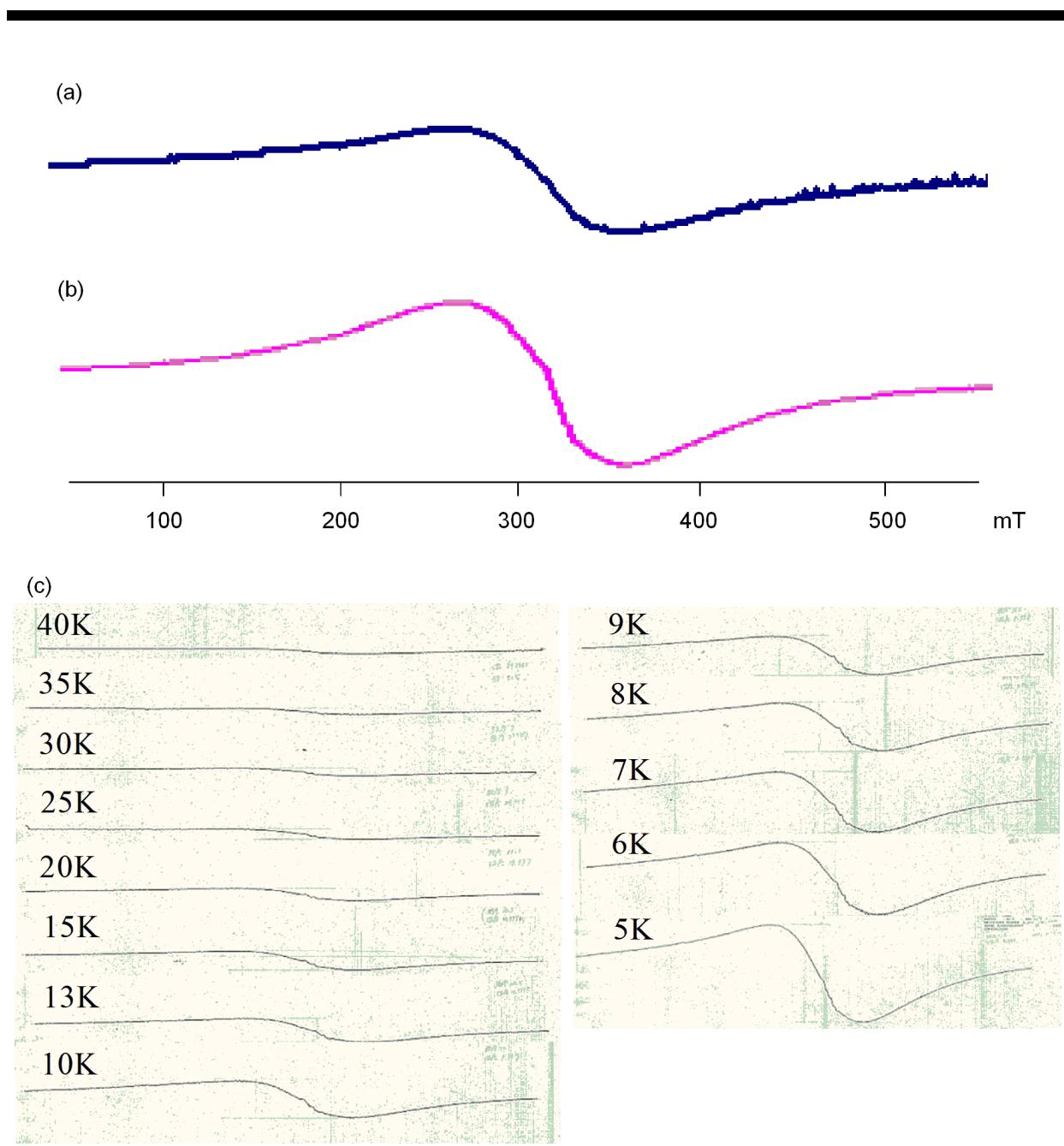
**Figure S6.** ESR spectra of  $\mathbf{1}^{2+} \cdot 2\text{PF}_6^-$  at 7 K in (a) the solid state and (b) a frozen solution of  $\text{CH}_3\text{CN}$  and (c) VT measurements of the solid sample.
