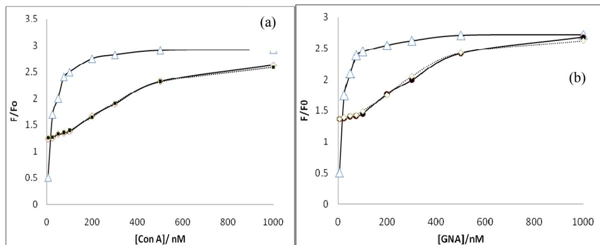
**Figure 4.** Rate of fluorescent gain from Ru(II)-carbohydrate-BBV upon addition of lectin; **1** ( ), **2** (◊) and **3** (◻) at  $\lambda_{\max} = 645$  nm. Concentration of  $\Delta$ complex **1** =  $1.0 \times 10^{-5} : 2.0 \times 10^{-4}$  M of BBV; Concentration of complex **2-3** =  $1.0 \times 10^{-5} : 2.0 \times 10^{-4}$  M of BBV
