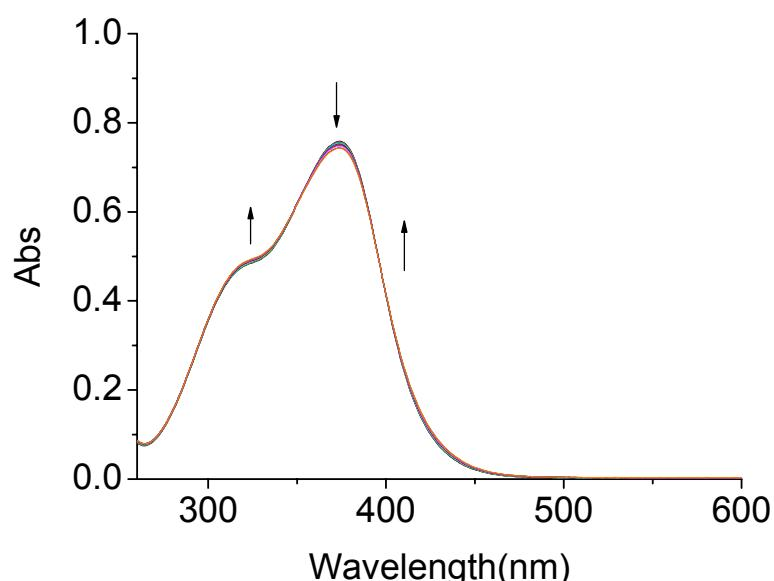
**Figure S11.** UV-Visible spectral changes of **1** ( $4.12 \times 10^{-5}$  M) upon addition of  $\text{SCN}^-$  as a tetrabutylammonium salt in  $\text{CH}_3\text{CN} / 3\%$  DMSO.
