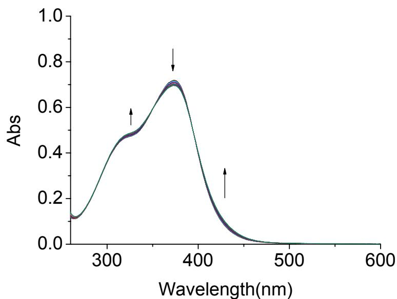
**Figure S12.** UV-Visible spectral changes of **1** ( $4.12 \times 10^{-5}$  M) upon addition of  $\text{HP}_2\text{O}_7^{3-}$  as a tetrabutylammonium salt in  $\text{CH}_3\text{CN} / 3\%$  DMSO.
