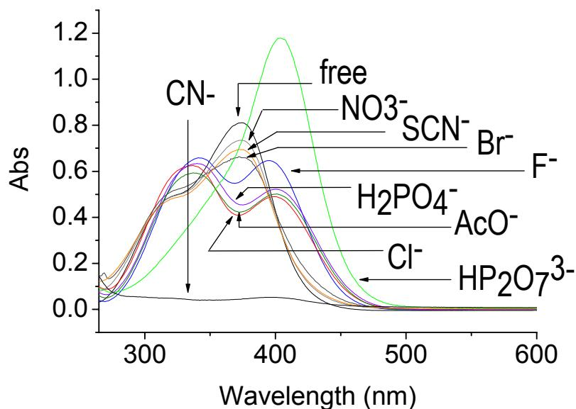
**Figure S22.** UV-Visible spectra of **1** ( $4.12 \times 10^{-5}$  M) with various anions where  $[F^-] = 3.80 \times 10^{-4}$  M,  $[Cl^-] = 9.19 \times 10^{-4}$  M,  $[Br^-] = 3.72 \times 10^{-4}$  M,  $[AcO^-] = 6.77 \times 10^{-4}$  M,  $[NO_3^-] = 6.83 \times 10^{-4}$  M,  $[H_2PO_4^-] = 6.76 \times 10^{-4}$  M,  $[SCN^-] = 3.85 \times 10^{-4}$  M,  $[HP_2O_7^{3-}] = 4.46 \times 10^{-4}$  M, and  $[CN^-] = 6.63 \times 10^{-4}$  M in CH<sub>3</sub>CN / 3% DMSO.
