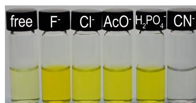
**Figure S23.** Color changes of **1** ( $1.03 \times 10^{-3}$  M) in the presence of anions (20 equiv, respectively) in CH<sub>3</sub>CN / 3% DMSO.
