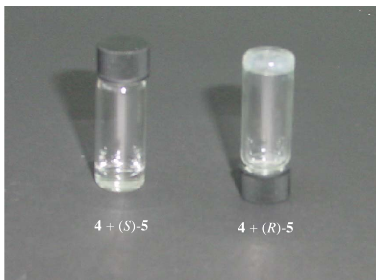
Figure S4. Gel from mixing of calix[4]arene 4 and amine ( R )- 5 (right) in 1,2-dichloroethane, and clear solution from mixing of calix[4]arene 4 and amine ( S )- 5 (left) in 1,2-dichloroethane.
