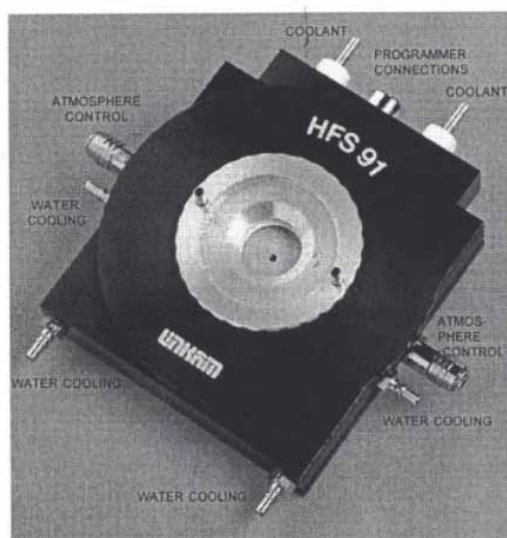
Fig.s1. Sketch photos of the low-temperature stage connections with Raman instruments.
