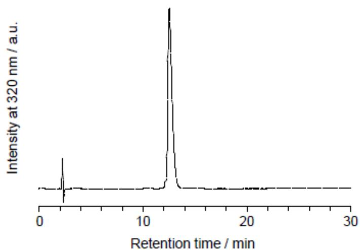
**Fig. S6** HPLC profile of apo-ASP. ASP was analyzed by reversed phase HPLC on Chemcobond 5-ODS-H (4.6 mm × 150 mm, Chemco Scientific Co., Ltd.) with a 30-min linear gradient of 25-70% acetonitrile/aqueous 0.1% TFA at a flow rate of 1 mL/min.
