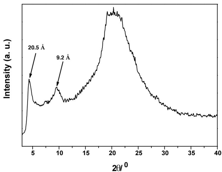
**Fig. S6** X-ray diffractogram of the xerogel of sample **1** prepared from cyclohexane ( $9.9 \times 10^{-3} \text{ mol dm}^{-3}$ ).
