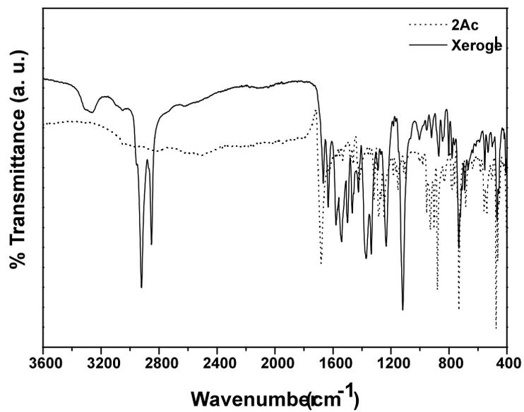
**Fig. S8** FT-IR spectra of 2Ac and xerogel of sample **1** ( $9.9 \times 10^{-3} \text{ mol dm}^{-3}$ ) prepared in cyclohexane.
