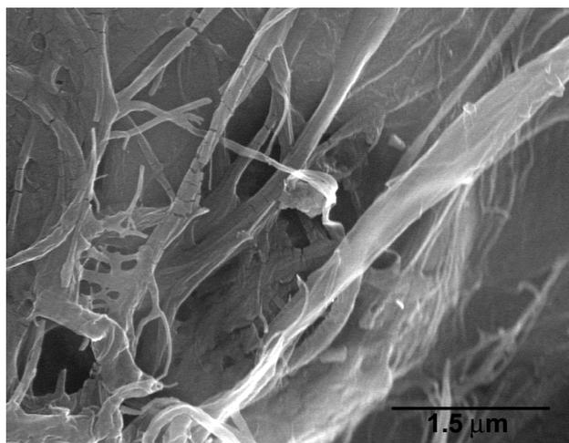
**Fig. S5** SEM image of xerogel of **1** ( $9.9 \times 10^{-3} \text{ mol dm}^{-3}$ ) prepared in cyclohexane.
