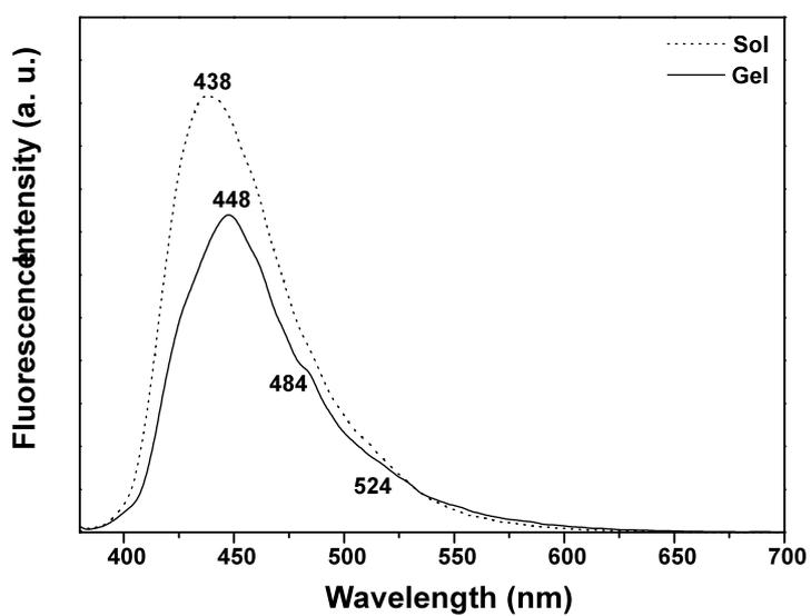
**Fig. S4** Fluorescence spectra of the sample **1** in the gel (25 °C) state and in the sol (50 °C) state prepared from cyclohexane ( $9.9 \times 10^{-3} \text{ mol dm}^{-3}$ ).
