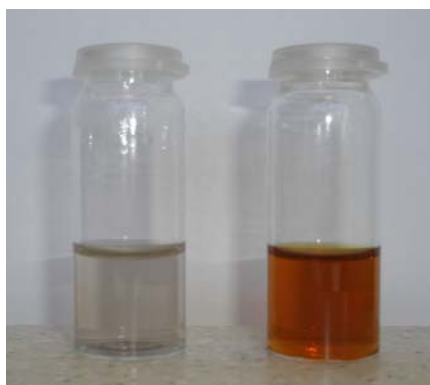
Figure S3. Silver nitrate solution at pH = 9 after bubbling with H 2 for 10 mins; left: without phosphonated calixarene, right: with 0.05 mM phosphonated calix[4]arene.
