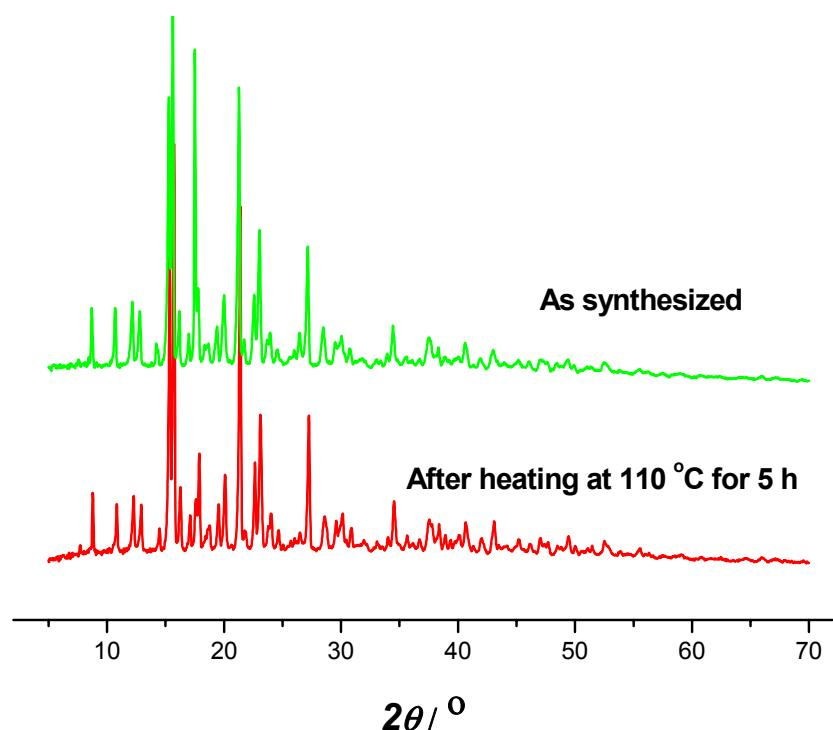
**Figure S6.** Powder X-ray diffraction patterns for compound **1**.
