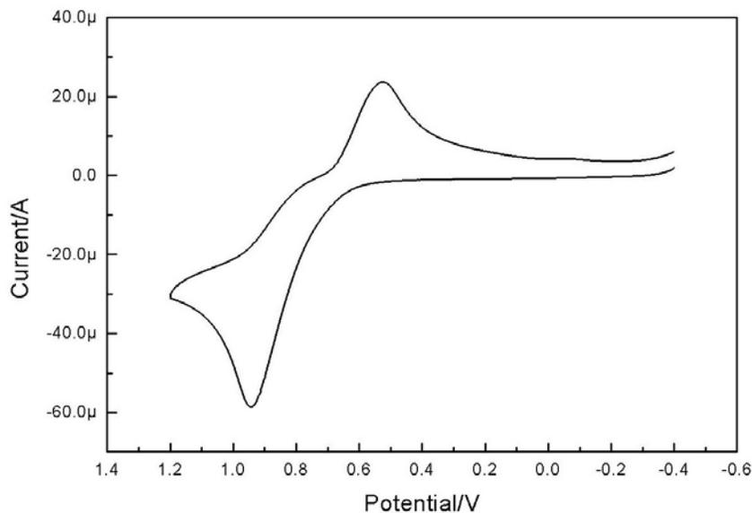
**Figure S15.** Cyclic voltammogram of **8** (4-nitrocatechol, 2 mM) in MeOH. NaNO<sub>3</sub> (0.15 M) was used as the supporting electrolyte. Working electrode: glassy carbon electrode; scan rate: 100 mV/s; reference electrode: Ag/AgCl.  $E_{pa} = 0.91$  V;  $E_{pc} = 0.54$  V.
