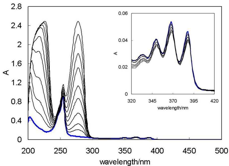
**Figure S27.** Absorption spectra of **1** (5.1 μM) and **2** (0 – 1.1 mM) in MeOH. The blue spectrum was taken in the absence of **2**. The zoom shot between 320 nm and 420 nm is shown in the inset.
