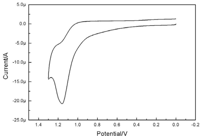
**Figure S7.** Cyclic voltammogram of **1** (0.3 mM) in MeOH. NaNO<sub>3</sub> (0.15 M) was used as the supporting electrolyte. Working electrode: glassy carbon electrode; scan rate: 100 mV/s; reference electrode: Ag/AgCl.  $E_{pa} = 1.16$  V.
