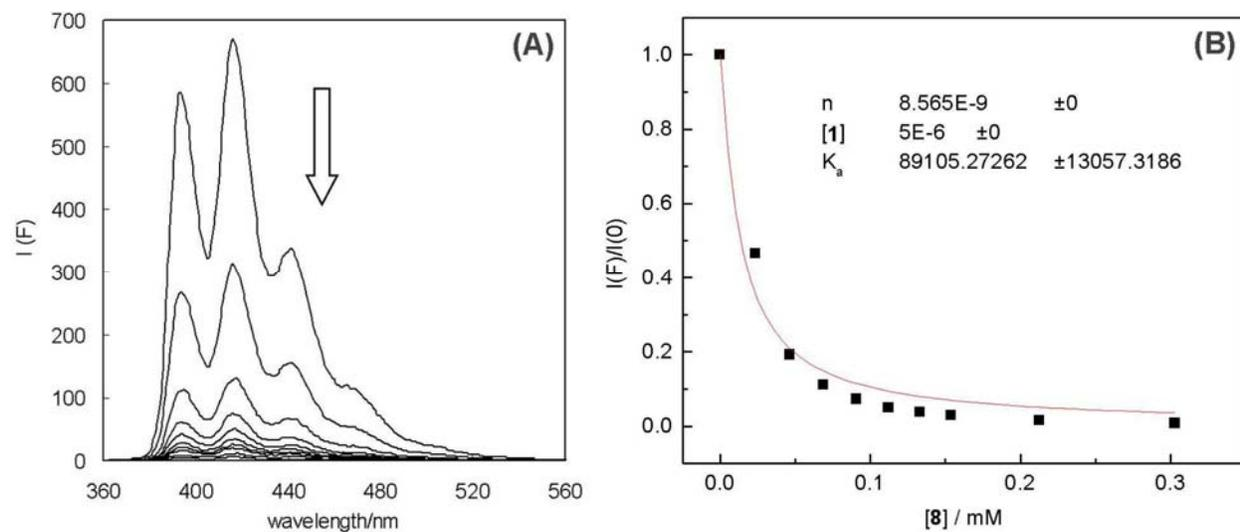
**Figure S24.** (A) Fluorescence spectral change of **1** ( $5.1 \mu\text{M}$ ,  $\lambda_{\text{ex}} = 350 \text{ nm}$ ) in MeOH with increasing concentration of **8** (0 – 0.3 mM). (B) Relative fluorescence intensity at 416 nm vs. **[8]**. The solid line is a theoretical fitting curve using a 1:1 binding isotherm.
