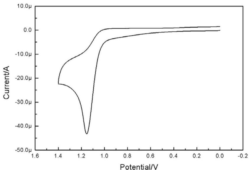
**Figure S8.** Cyclic voltammogram of anthracene (2 mM) in MeOH. NaNO<sub>3</sub> (0.15 M) was used as the supporting electrolyte. Working electrode: glassy carbon electrode; scan rate: 100 mV/s; reference electrode: Ag/AgCl.  $E_{pa} = 1.15$  V.
