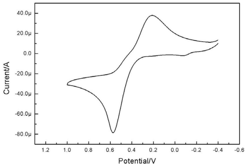
**Figure S13.** Cyclic voltammogram of **6** (4-methoxycatechol) in MeOH.  $\text{NaNO}_3$  (0.15 M) was used as the supporting electrolyte. Working electrode: glassy carbon electrode; scan rate: 100 mV/s; reference electrode: Ag/AgCl.  $E_{pa} = 0.57$  V;  $E_{pc} = 0.21$  V.
