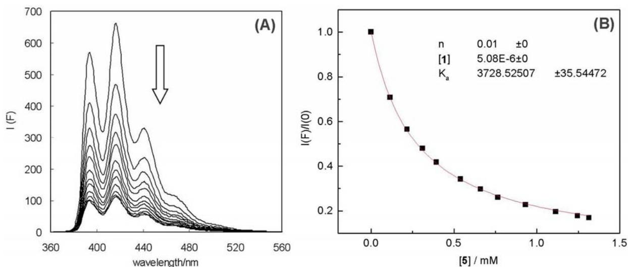
**Figure S21.** (A) Fluorescence spectral change of **1** ( $5.1 \mu\text{M}$ ,  $\lambda_{\text{ex}} = 350 \text{ nm}$ ) in MeOH with increasing concentration of **5** (0 – 1.3 mM). (B) Relative fluorescence intensity at 416 nm vs. **[5]**. The solid line is a theoretical fitting curve using a 1:1 binding isotherm.
