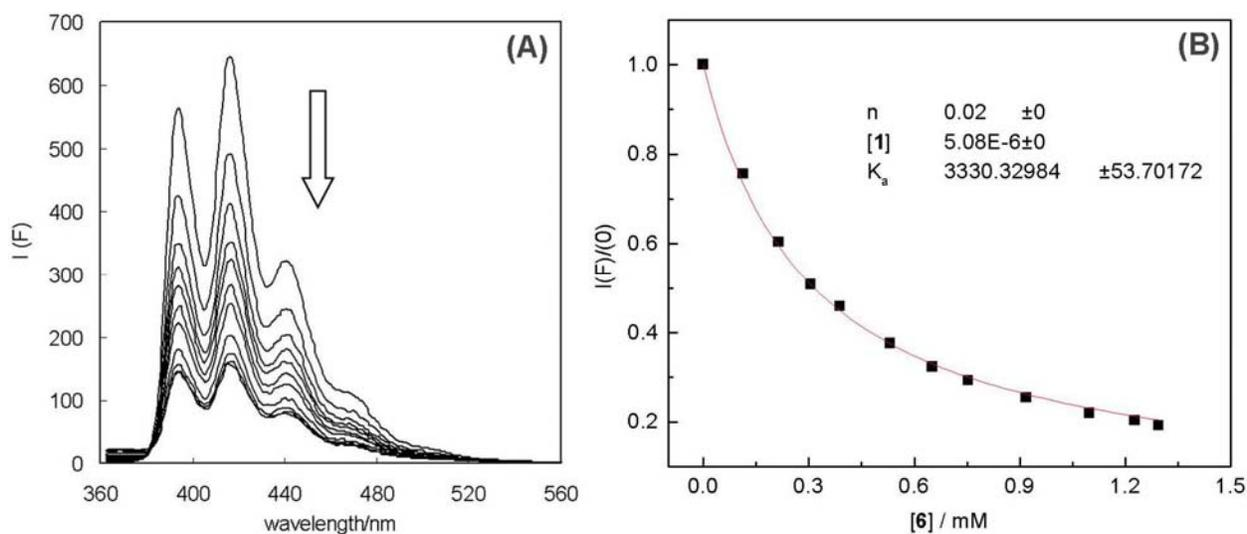
**Figure S22.** (A) Fluorescence spectral change of **1** ( $5.1 \mu\text{M}$ ,  $\lambda_{\text{ex}} = 350 \text{ nm}$ ) in MeOH with increasing concentration of **6** (0 – 1.3 mM). (B) Relative fluorescence intensity at 416 nm vs. **[6]**. The solid line is a theoretical fitting curve using a 1:1 binding isotherm.
