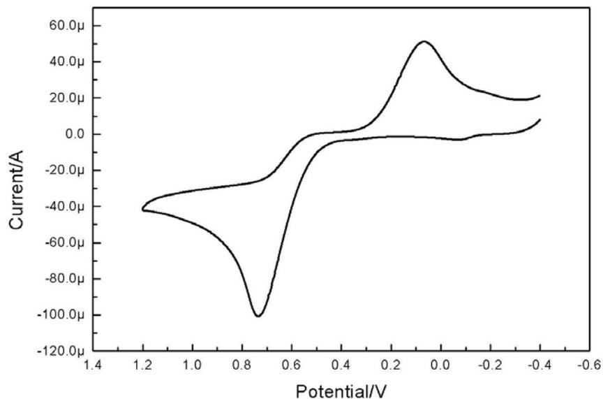
**Figure S17.** Cyclic voltammogram of hydroquinone (3 mM) in MeOH. NaNO<sub>3</sub> (0.15 M) was used as the supporting electrolyte. Working electrode: glassy carbon electrode; scan rate: 100 mV/s; reference electrode: Ag/AgCl.  $E_{pa} = 0.74$  V;  $E_{pc} = 0.07$  V.
