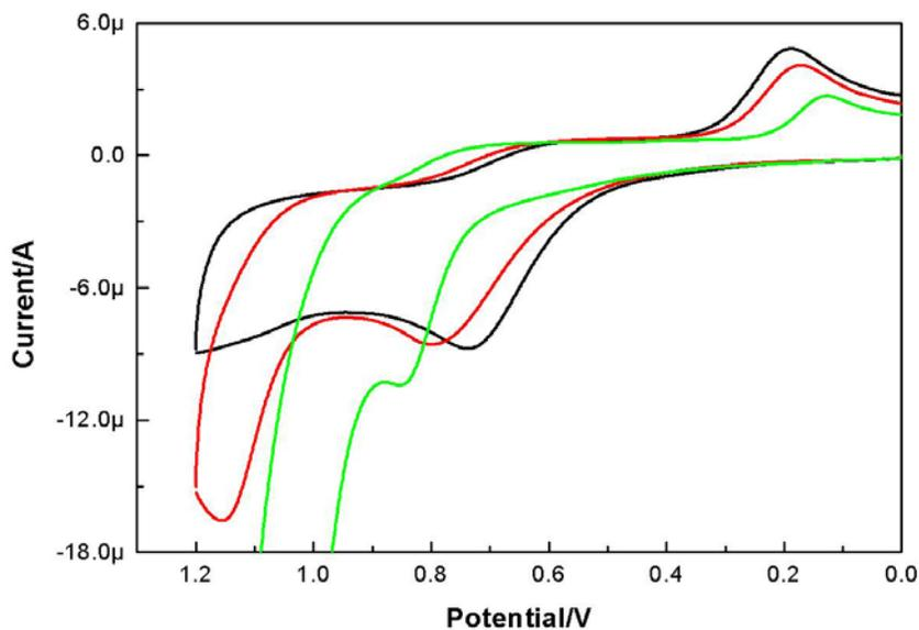
**Figure S18.** Cyclic voltammogram of **3** (0.2 mM) in MeOH in the presence of 0 (black), 0.1 mM (red), and 4.9 mM (green) of **1**. NaNO<sub>3</sub> (0.15 M) was used as the supporting electrolyte. Working electrode: glassy carbon electrode; scan rate: 100 mV/s; reference electrode: Ag/AgCl.
