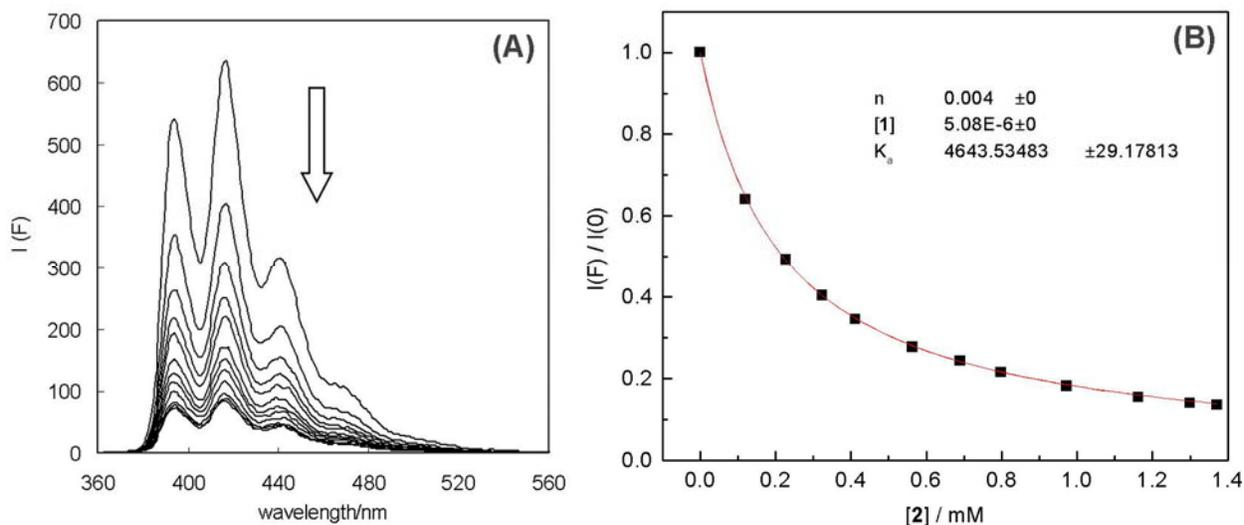
**Figure S19.** (A) Fluorescence spectral change of **1** (5.1  $\mu\text{M}$ ,  $\lambda_{\text{ex}} = 350 \text{ nm}$ ) in MeOH with increasing concentration of **2** (0 – 1.4 mM). (B) Relative fluorescence intensity at 415 nm vs. **[2]**. The solid line is a theoretical fitting curve using a 1:1 binding isotherm.
