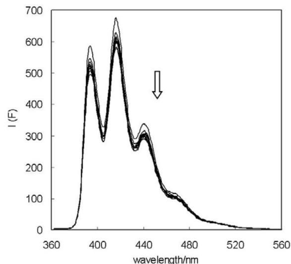
**Figure S26.** (A) Fluorescence spectral change of **1** ( $5.1 \mu\text{M}$ ,  $\lambda_{\text{ex}} = 350 \text{ nm}$ ) in MeOH with increasing concentration of hydroquinone ( $0 - 1.3 \text{ mM}$ ).
