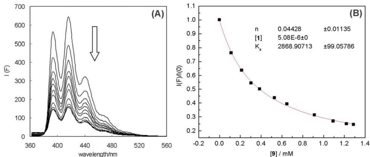
**Figure S25.** (A) Fluorescence spectral change of **1** ( $5.1 \mu\text{M}$ ,  $\lambda_{\text{ex}} = 350 \text{ nm}$ ) in MeOH with increasing concentration of **9** ( $0 - 1.3 \text{ mM}$ ). (B) Relative fluorescence intensity at  $416 \text{ nm}$  vs.  $[\mathbf{9}]$ . The solid line is a theoretical fitting curve using a 1:1 binding isotherm.
