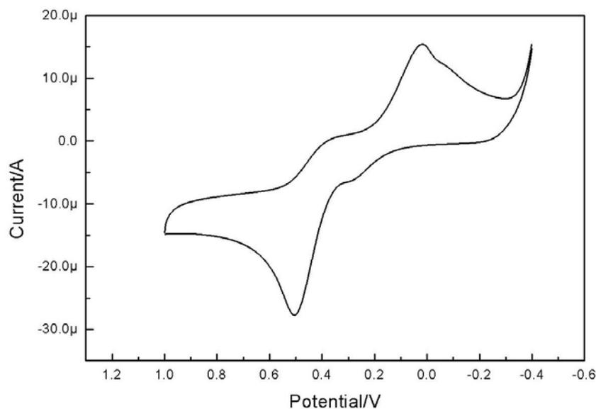
**Figure S16.** Cyclic voltammogram of **9** (1,2,4-benzenetriol, 0.3 mM) in MeOH. NaNO<sub>3</sub> (0.15 M) was used as the supporting electrolyte. Working electrode: glassy carbon electrode; scan rate: 100 mV/s; reference electrode: Ag/AgCl.  $E_{pa} = 0.50$  V;  $E_{pc} = 0.03$  V.
