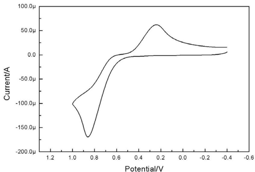
**Figure S9.** Cyclic voltammogram of **2** (catechol, 5 mM) in MeOH. NaNO<sub>3</sub> (0.15 M) was used as the supporting electrolyte. Working electrode: glassy carbon electrode; scan rate: 100 mV/s; reference electrode: Ag/AgCl. E<sub>pa</sub> = 0.84 V; E<sub>pc</sub> = 0.24 V.
