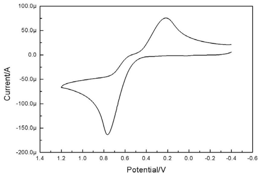
**Figure S12.** Cyclic voltammogram of **5** (4-methylcatechol, 5 mM) in MeOH. NaNO<sub>3</sub> (0.15 M) was used as the supporting electrolyte. Working electrode: glassy carbon electrode; scan rate: 100 mV/s; reference electrode: Ag/AgCl.  $E_{pa} = 0.77$  V;  $E_{pc} = 0.22$  V.
