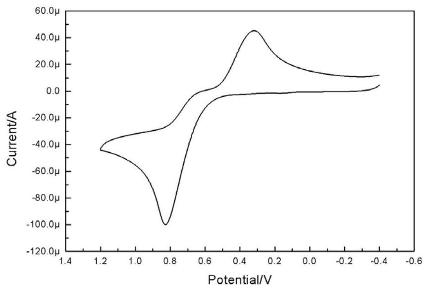
**Figure S11.** Cyclic voltammogram of **4** (4-chlorocatechol, 3 mM) in MeOH. NaNO<sub>3</sub> (0.15 M) was used as the supporting electrolyte. Working electrode: glassy carbon electrode; scan rate: 100 mV/s; reference electrode: Ag/AgCl.  $E_{pa} = 0.83$  V;  $E_{pc} = 0.32$  V.
