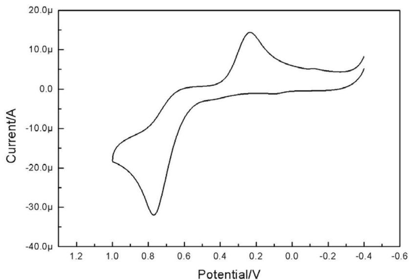
**Figure S10.** Cyclic voltammogram of **3** (4-fluorocatechol, 0.6 mM) in MeOH. NaNO<sub>3</sub> (0.15 M) was used as the supporting electrolyte. Working electrode: glassy carbon electrode; scan rate: 100 mV/s; reference electrode: Ag/AgCl. E<sub>pa</sub> = 0.77 V; E<sub>pc</sub> = 0.23 V.
