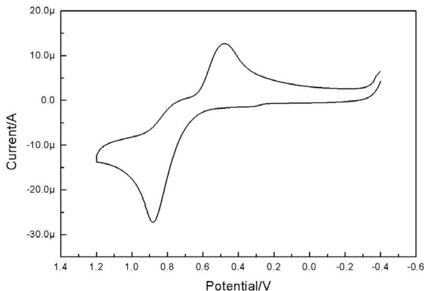
**Figure S14.** Cyclic voltammogram of **7** (4-cyanocatechol, 0.9 mM) in MeOH.  $\text{NaNO}_3$  (0.15 M) was used as the supporting electrolyte. Working electrode: glassy carbon electrode; scan rate: 100 mV/s; reference electrode: Ag/AgCl.  $E_{pa} = 0.88$  V;  $E_{pc} = 0.48$  V.
