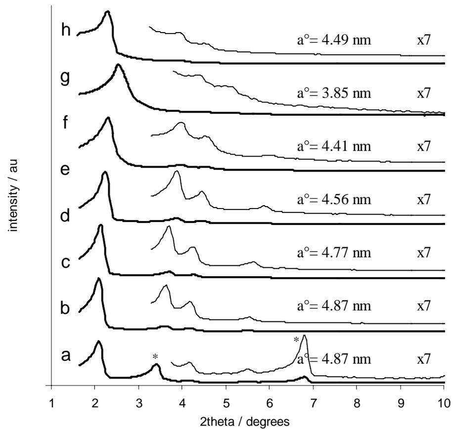
**Fig.S1.** Powder XRD patterns: COK-11 as-synthesised (a), leached (b), calcined at 573 K (c), calcined at 898 K (d), calcined at 898 K and stored 3 years at room temperature (e), calcined at 1273 K (f) and calcined at 898 K and hydrothermally treated for 24 h at 373 K (g). Signals originating from CTAB crystals are marked with an \*.
