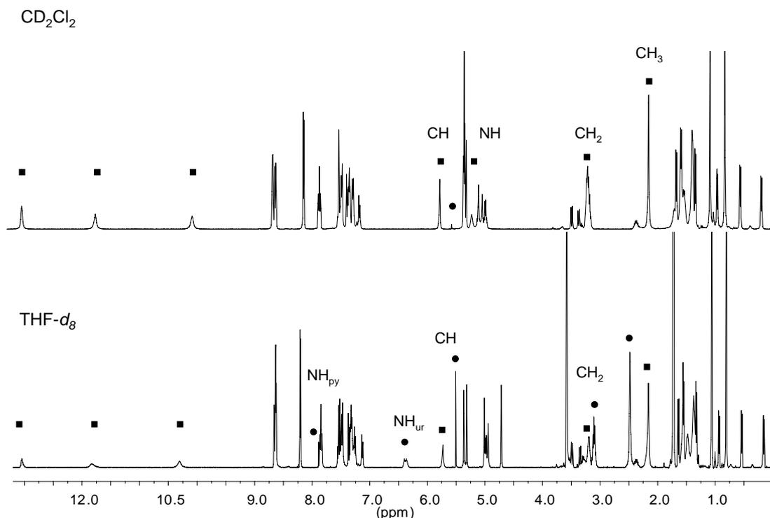
Comparison of the  $^1\text{H-NMR}$  spectra of “tpy~TIPNO~UPy”(5) in  $\text{CD}_2\text{Cl}_2$  and  $\text{THF-d}_8$  shows the influence of the solvent on the tautomeric equilibrium. Besides the dimeric form of 4[1H]-pyrimidinone (■) also the monomeric form of 4[3H]-pyrimidinone (●) can be observed.<sup>[9]</sup>
