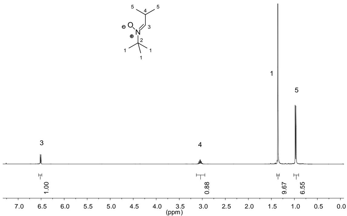
$^1\text{H-NMR}$  spectrum of *N*-tert-butyl- $\alpha$ -iso-propylnitrone (400 MHz,  $\text{CDCl}_3$ ).
