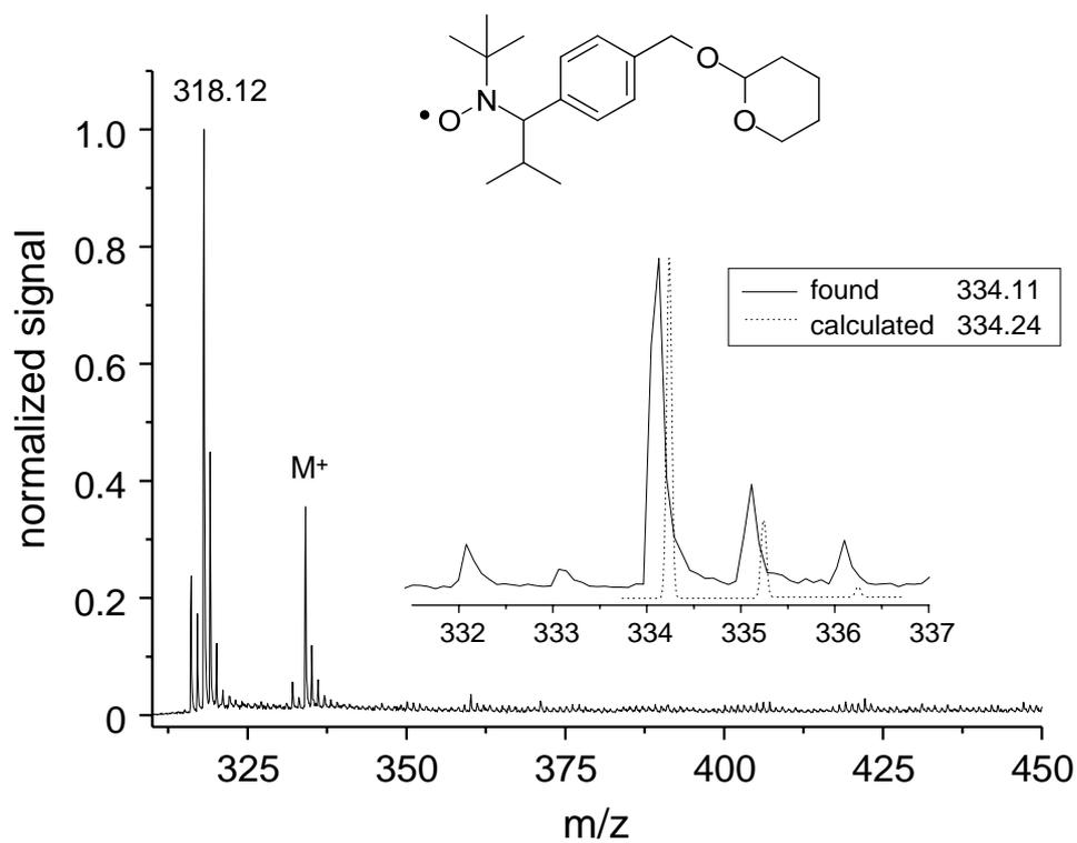
*MALDI-TOF MS spectrum of functional TIPNO showing abstraction of oxygen as well as of hydrogen (matrix: dithranol).*
