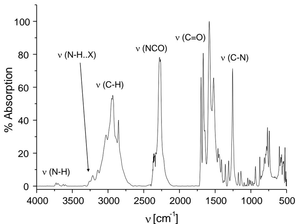
*FT-IR spectrum of building block 4 shows characteristic absorption bands for isocyanate ( $N=C=O$ -valence) and for the hydrogen bonding ( $N-H..X$ -valence).*
