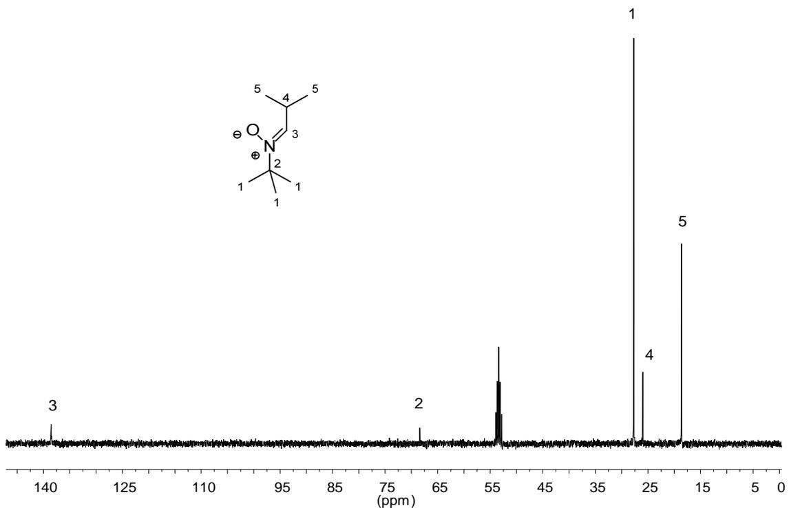
$^{13}\text{C-NMR}$  spectrum of *N*-tert-butyl- $\alpha$ -iso-propylnitrone (100 MHz,  $\text{CD}_2\text{Cl}_2$ ).
