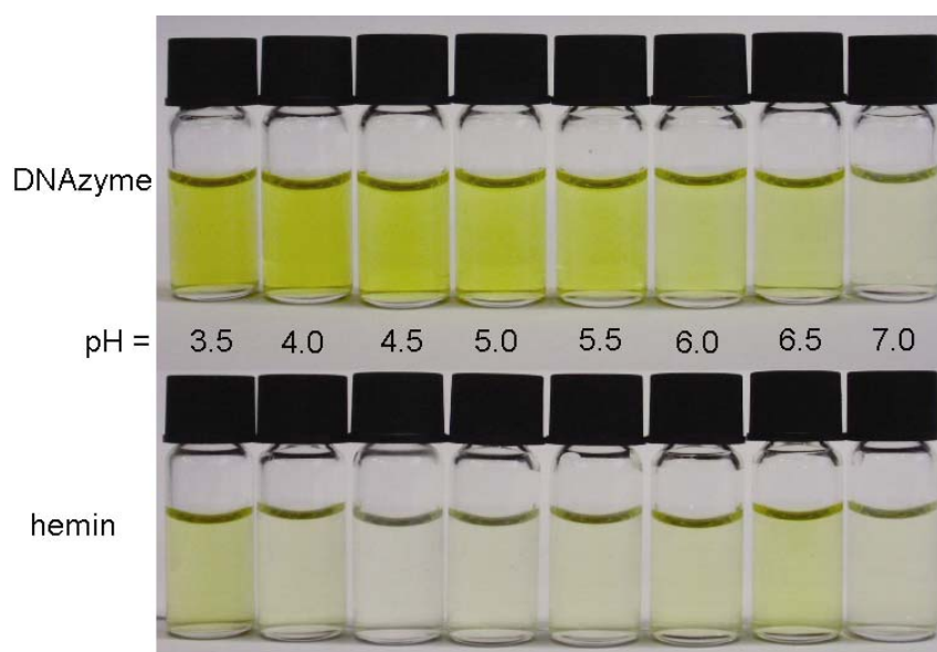
Fig. S1 Effect of pH of the reaction solution on the DNAzyme activity and the background imparted by hemin catalysis.
