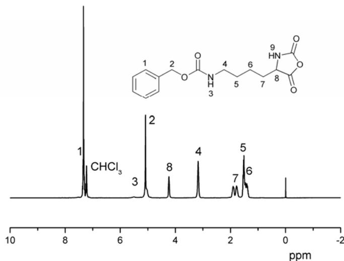
**Fig. 3** <sup>1</sup>H NMR spectrum of **ZLys-NCA**
