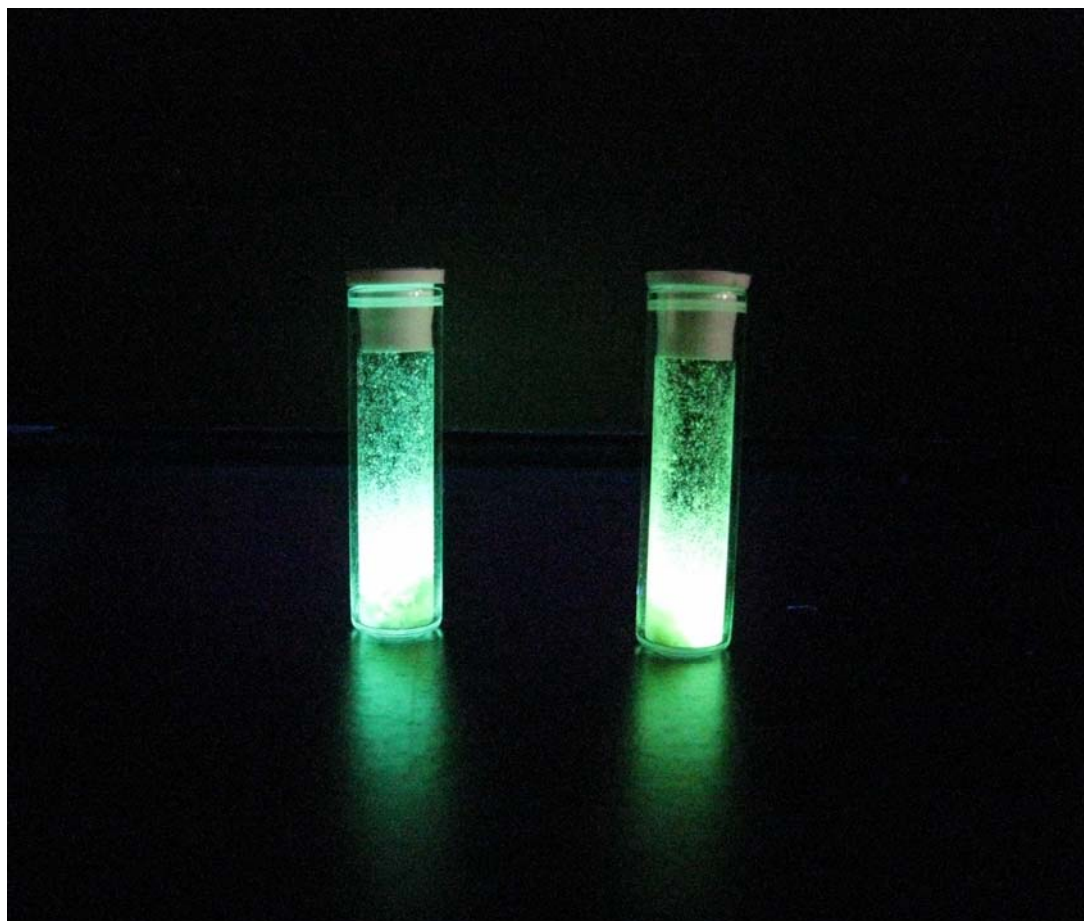
Fig. S8. The solid-state emission colours of (a) Pt-Ge and (b) Pt-O upon UV irradiation. In each case, intense green emission was observed on the wall with a low density of the emitter. Near-white light can be observed at the centre of the sample vials where a very high density of the emitter results in an extremely intense light emission.
