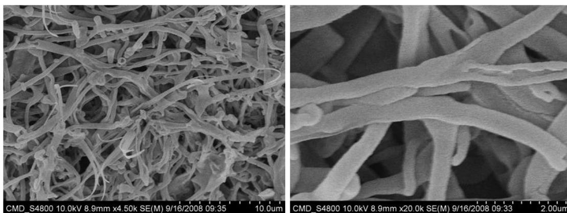
**Figure S6.** Titanium oxide nanofibers made with SMC (Mw 250K) nanofibers as templates.
