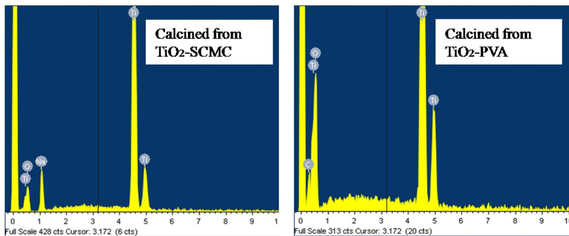
**Figure S7.** Element analysis of titanium oxide nanofibers made from SCMC and PVA, as measured by energy dispersive X-ray (EDX) microanalysis. The presence of Na from SCMC-made nanofibers is clearly seen with a weight percentage of 11.42 %. The first strong unlabelled signals are from the Beryllium (Be) internal standard.
