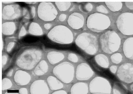
**Figure S3.** STEM image of a PVA nanofiber obtained from freezing 0.1 wt % PVA (Mw 89,000-98,000) in liquid nitrogen. Scale bar: 600 nm.
