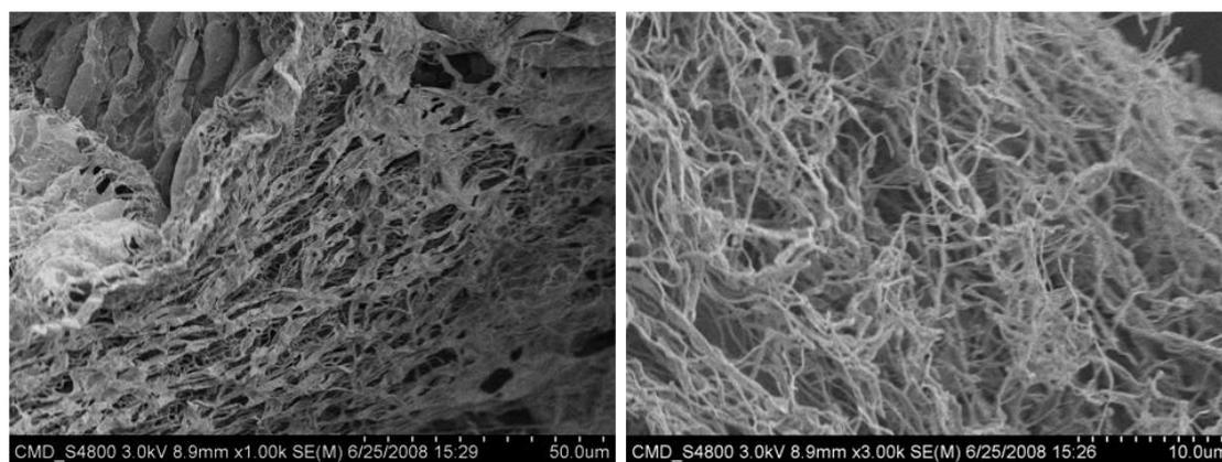
**Figure S2.** Porous structure of PVA (Mw 89-98K) processed from the 0.5 wt % aqueous solution. Part of it was nanofiber structure (image on the right).
