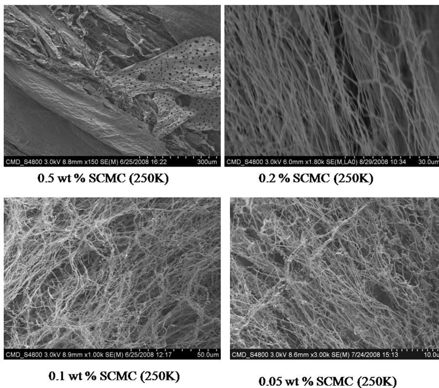
**Figure S1.** Porous structures of aqueous SCMC (Mw 250K) solutions with different concentrations frozen in liquid nitrogen and then freeze dried. Freezing dilute solutions led to the formation of nanofibers.
