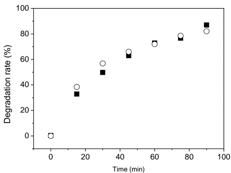
**Figure S5.** Degradation rate of Rhodamine B in water under UV irradiation (254 nm) using titania as the photocatalyst: TiO<sub>2</sub> nanofibers (○) and P25 (■). The initial concentration of Rhodamine B was 10 mg/L.
