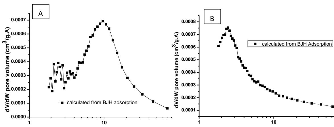
**Figure S4.** (A) Pore size distribution of titania nanofibers made using PVA as template. This material has a BET surface area of  $53.20 \text{ m}^2 \cdot \text{g}^{-1}$  and a mesopore size distribution around 10 nm. (B) Pore size distribution of titania powders P25 (Degussa). This commercial product exhibits a surface area of  $52.80 \text{ m}^2 \cdot \text{g}^{-1}$  (measured by us) or  $50 \pm 15 \text{ m}^2 \cdot \text{g}^{-1}$  (data from the provider).
