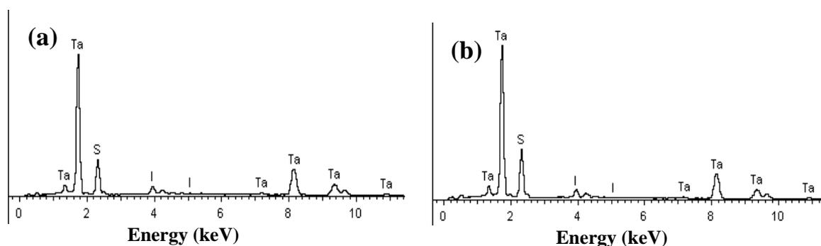
**Fig. S1.** EDX spectra of the products prepared with a 30 mg of iodine. (a) A single nanorod; (b) a piece of nanosheet.
