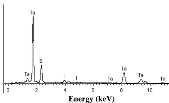
**Fig. S3.** EDX spectrum of the nanosheets prepared with a 120 mg of iodine.
