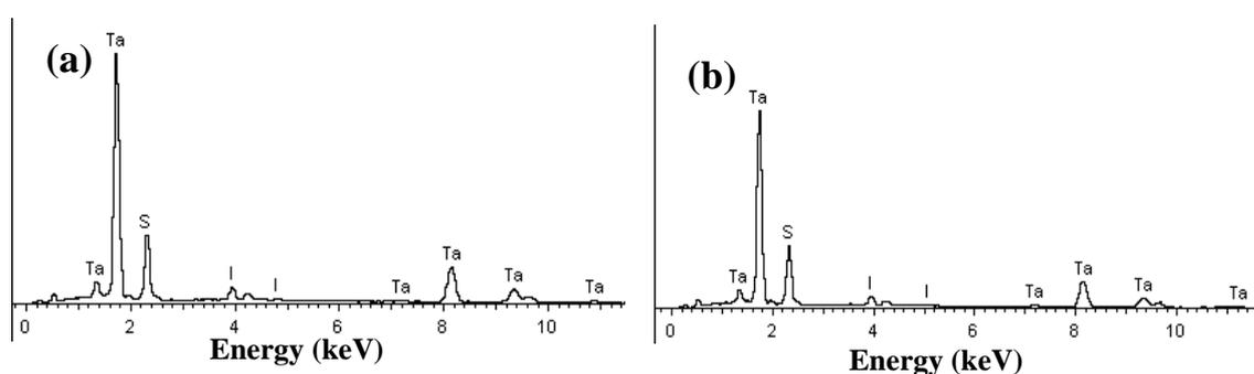
**Fig. S2.** EDX spectra of the products prepared with a 60 mg of iodine. (a) A single nanorod; (b) a piece of nanosheet.
