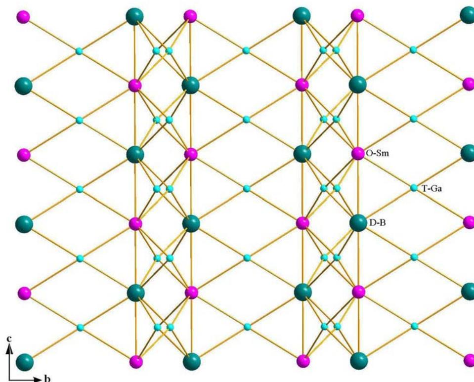
**Figure S2.** Simplified honeycomb-like open-framework of **1** along the *a* direction, where the dark yellow, turquoise and pink balls represent B<sub>12</sub> dodecaborate (D-B), GaS<sub>4</sub> tetrahedra (T-Ga) and SmS<sub>6</sub> octahedra (O-Sm), respectively.
