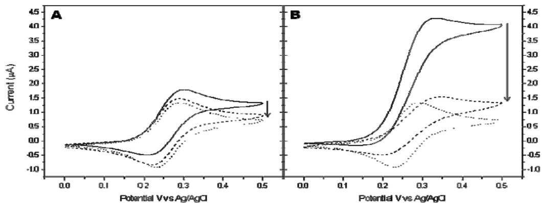
**Fig. S2** Cyclic voltammograms before (A) and after (B) the addition of biotin-dendrimer on the sensing surface with artificial wild type sample (solid line), or artificial mutant sample (single-base substitution in position 3459, dashed line), and without electrocatalysis (control, dotted line).
