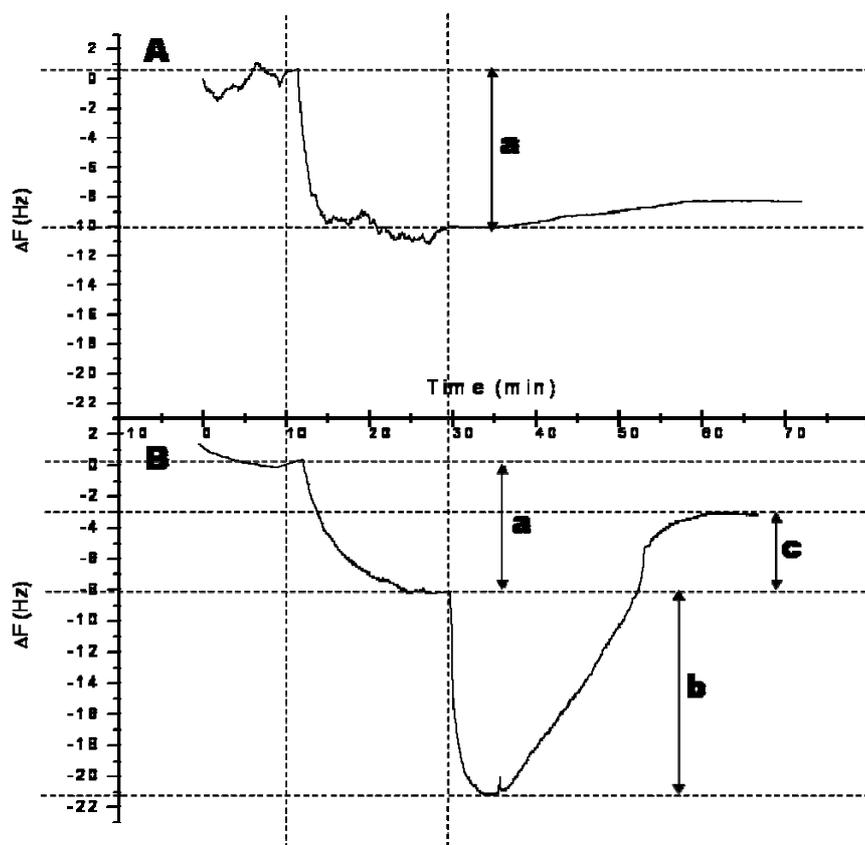
**Fig. S1** Frequency shift of Au-coated quartz crystal electrode, modified with biotin-tagged capture probe, after addition of target samples (10 min) and CEL I nuclease (30 min) with perfectly matched target (A) and single-base mismatched target (B). The data indicate target hybridization with capture probe (a), CEL I binding to the mismatched site (b), and release of cleaved fraction (c).
