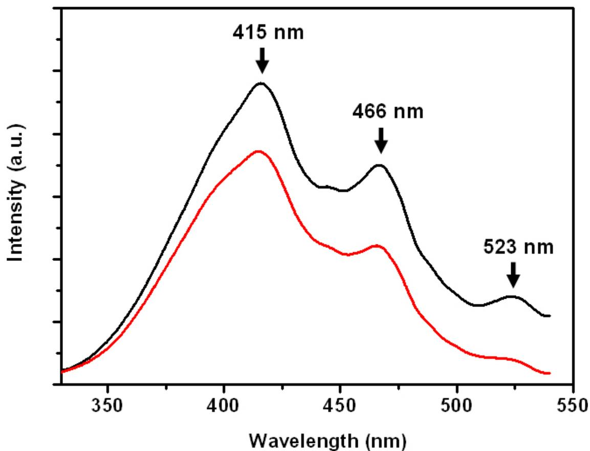
**Fig. S7** PL spectra of non-hollow hexagonal rod-shaped In<sub>2</sub>O<sub>3</sub> (red) and hollow elongated hexagonal-shaped In<sub>2</sub>O<sub>3</sub> (black) under excited wavelength of 280 nm at room temperature.
