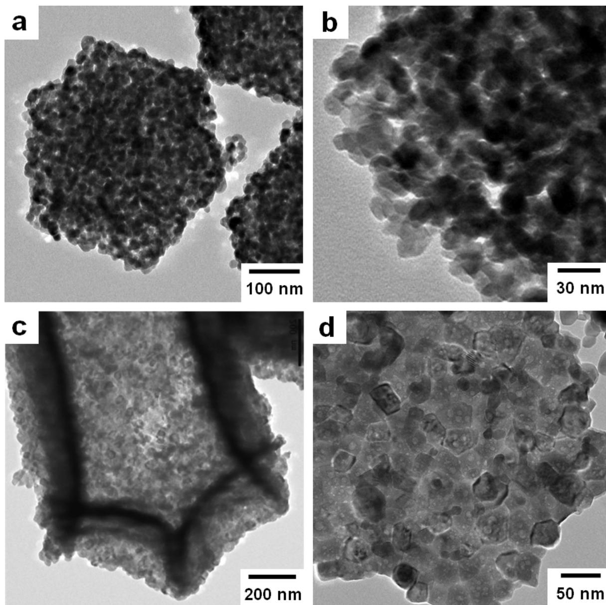
**Fig. S5** High magnification TEM images of (a, b) non-hollow hexagonal disk-shaped and (c, d) hollow elongated hexagon-shaped  $\text{In}_2\text{O}_3$ . The TEM images clearly show the polycrystalline structure.
