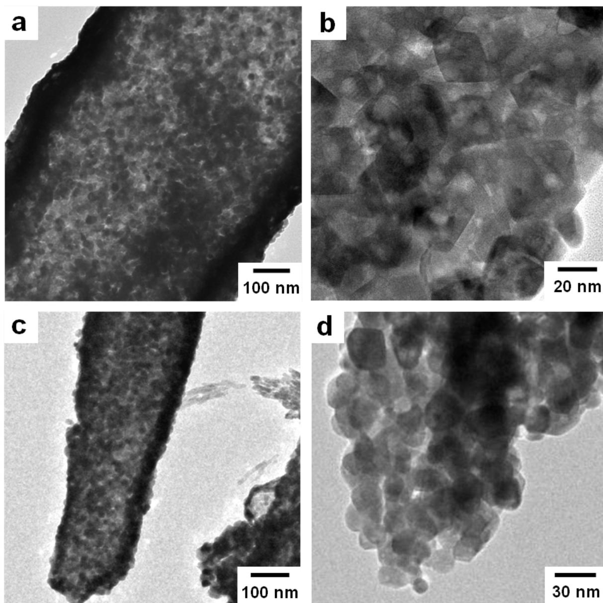
**Fig. S6** High magnification TEM images of (a, b) hollow ellipsoid-shaped and (c, d) hollow rod-shaped  $\text{In}_2\text{O}_3$ . The TEM images clearly show the polycrystalline structure.
