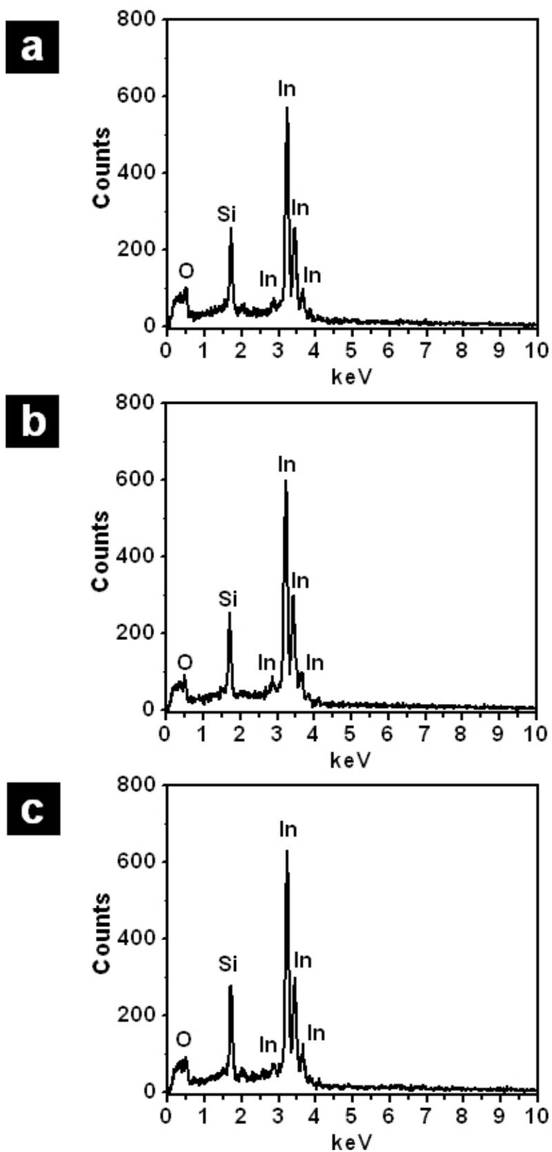
**Fig. S2** EDX spectra of (a) non-hollow hexagonal disk-shaped, (b) hollow ellipsoid-shaped, and (c) hollow rod-shaped  $\text{In}_2\text{O}_3$ .
