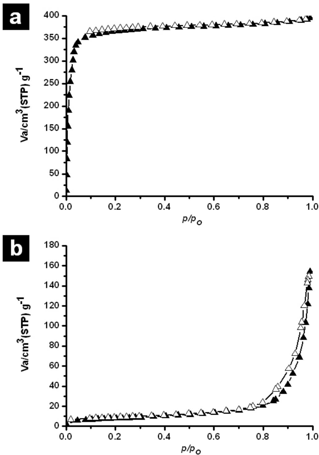
**Fig. S1** Nitrogen sorption isotherms at 77 K for (a) CPP-3 (Ref. S1) and (b) hexagonal rod-shaped  $\text{In}_2\text{O}_3$  (solid triangle, adsorption; open triangle, desorption).
