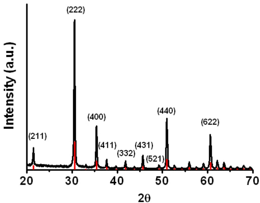
**Fig. S3** PXRD pattern of non-hollow hexagonal disk-shaped  $\text{In}_2\text{O}_3$ . Red sticks are the reported values of the cubic phase of  $\text{In}_2\text{O}_3$  (JCPDS Card No. 06-0416).
