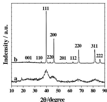
**Figure S1.** XRD patterns of (a) as-synthesized FeNiPt nanowires and (b) annealed at 823K for 1h.
