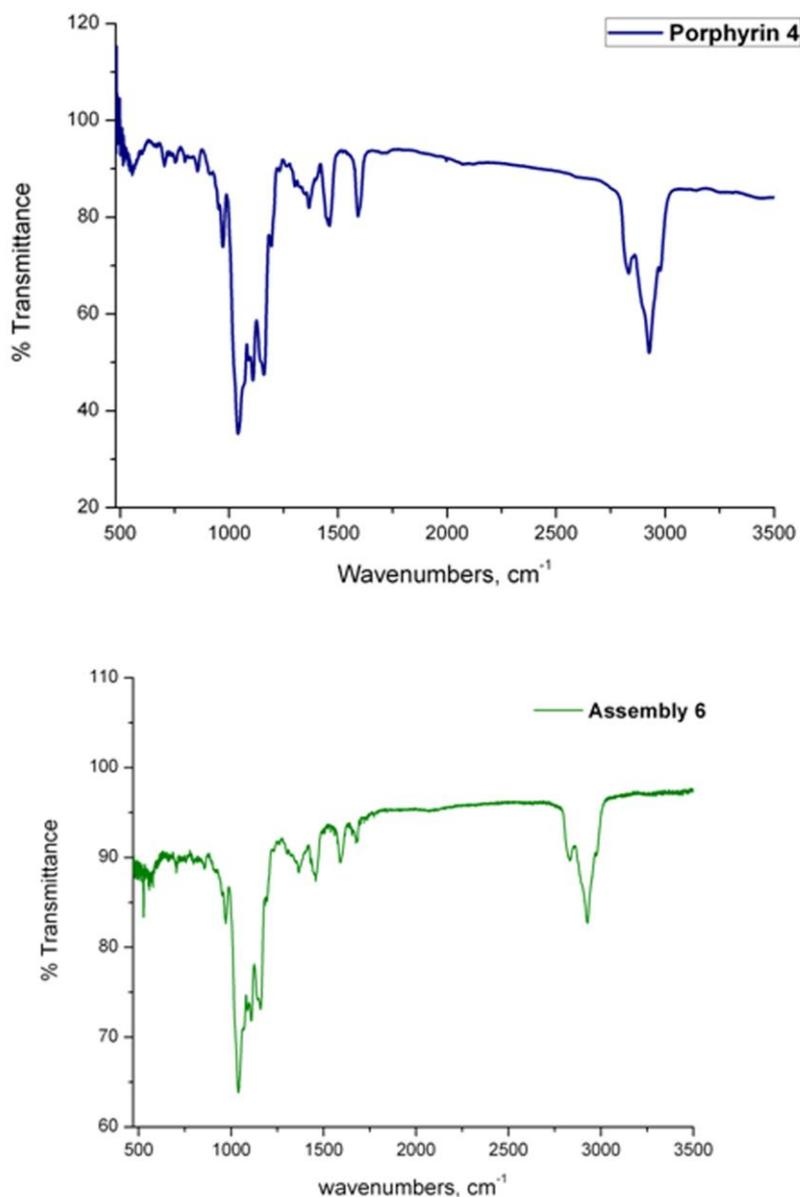
**Figure S1.** IR spectra of porphyrin **4** (top) and assembly **6** (bottom). Note the sharp peak at 527 cm<sup>-1</sup> which is a characteristic fullerene vibrational mode.<sup>5</sup>
