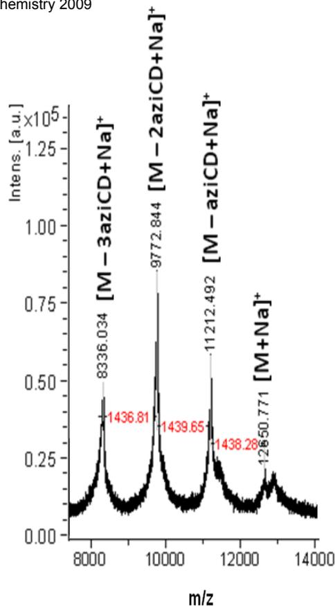
**Figure S13.** MALDI TOF-MS (DHB matrix) spectrum of porphyrin **4** (in the 7500-14000 Da region). The spectrum shows the parent peak at 12650.8 Da as well as fragmentation products ascribed to the sequential loss of the azido permethyl-β-cyclodextrin units.
