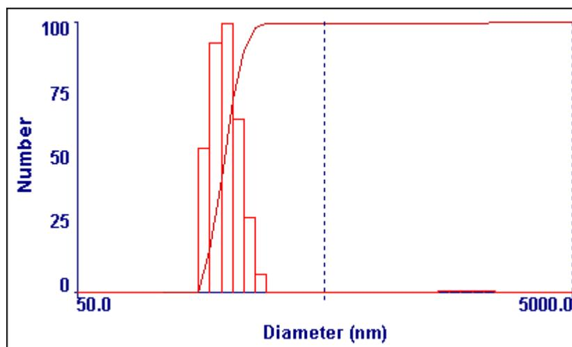
**Figure S3.** Multi-size distribution from dynamic light scattering measurements for assembly **6** ( $0.3 \times 10^{-6}$  M) in water. The intensity-weighted average particle diameter was  $D_h=263$ nm and broad particle distribution was observed.
