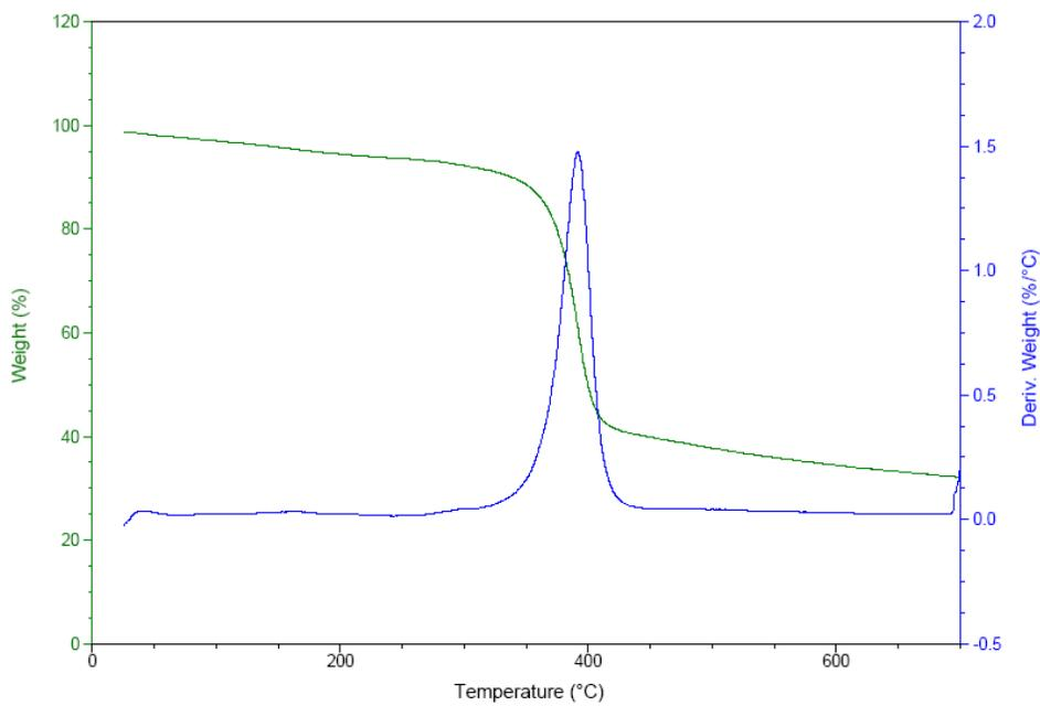
**Figure S6.** Thermogravimetric curve for assembly **6**.
