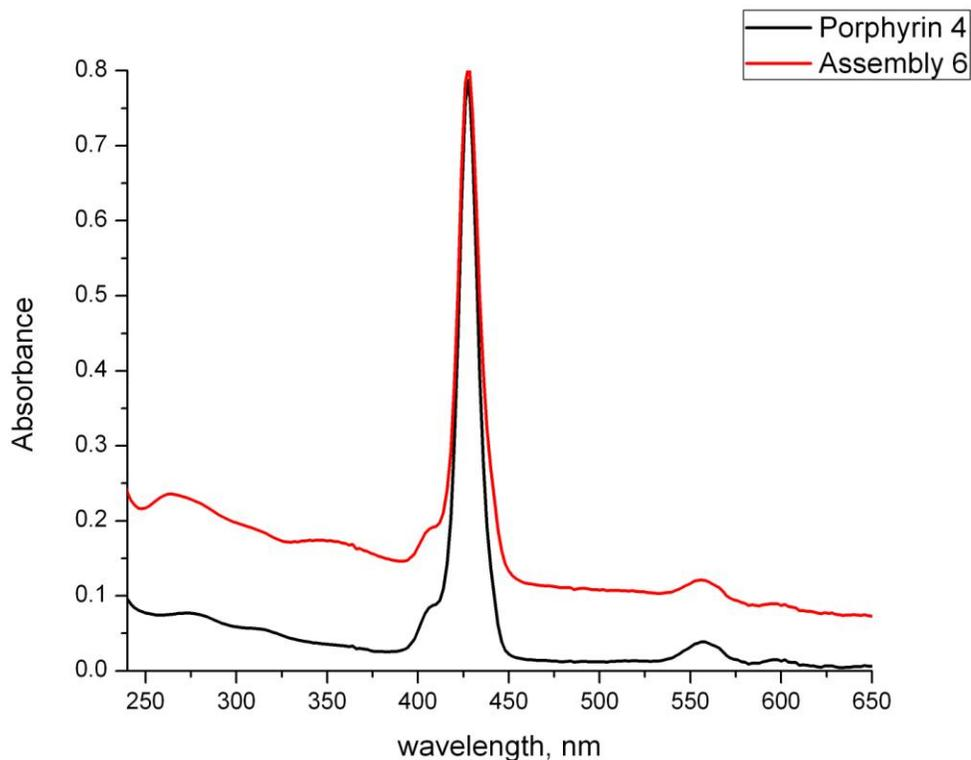
**Figure S2.** Electronic absorption spectra of porphyrin **4** (black line) and assembly **6** (red line) in water. Concentrations are  $3 \times 10^{-6}$  M.
