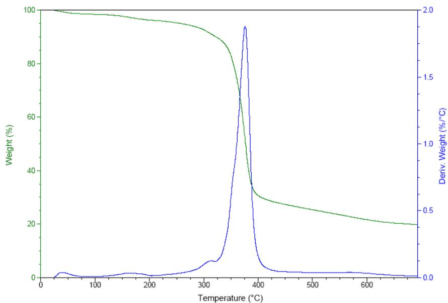
**Figure S5.** Thermogravimetric curve for porphyrin **4**.
