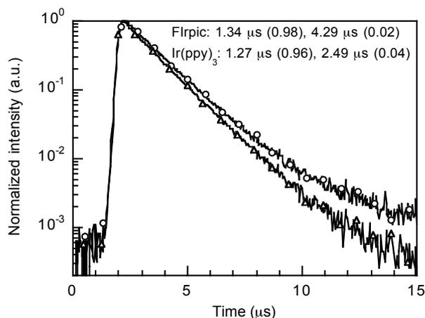
**Figure S-3.** Transient photoluminescence decay curves of CzTP/Firpic film (circles) and CzTP/Ir(ppy)<sub>3</sub> film (triangles) at room temperature.
