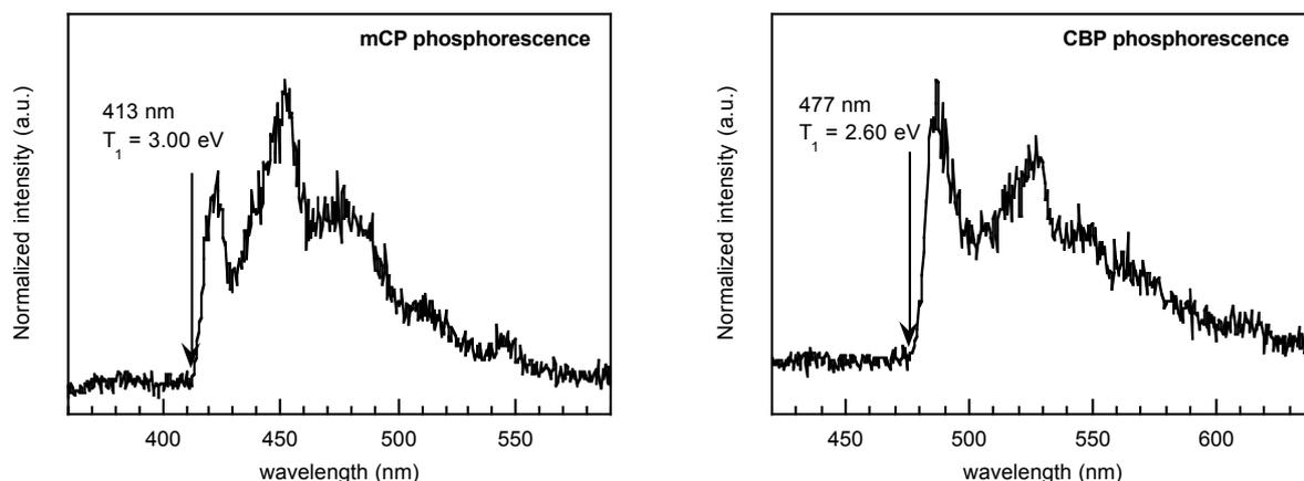
**Figure S-2.** Phosphorescent spectra of vacuum-deposited film of mCP (left) and CBP (right) at 4.2 K, measured by streak camera with a N<sub>2</sub> gas laser (337 nm) as an excitation light.
