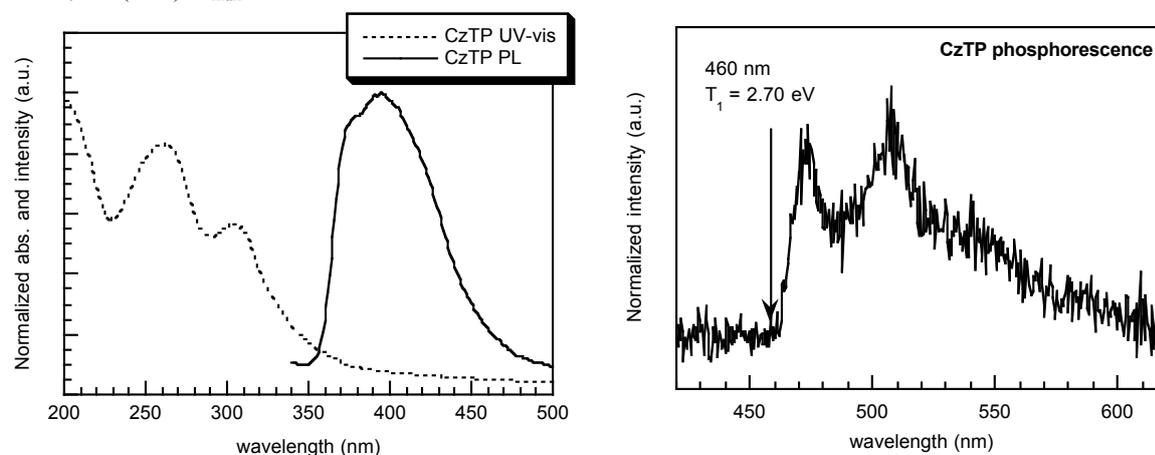
**Figure S-1.** UV-vis and PL spectra of vacuum deposited film of CzTP (left). Phosphorescent spectrum of vacuum-deposited film of CzTP at 4.2 K, measured by streak camera with a N<sub>2</sub> gas laser (337 nm) as an excitation light (right).
