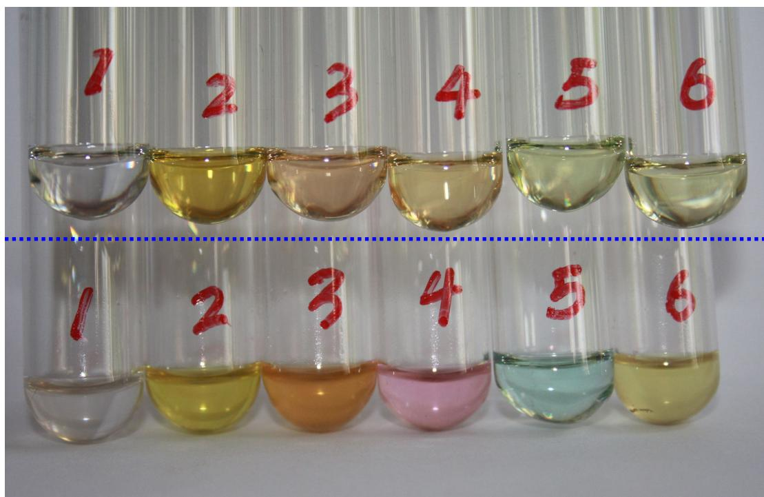
**ESI-Fig. 3** The upper samples show the indicators dissolved in benzene (1. benzene; 2. dimethyl yellow; 3. methyl red; 4. neutral red; 5. bromothymol blue; 6. thymol blue); the lower samples show complex (**1**) dissolved in benzene solution after addition of different indicators (1. blank [complex (**1**) dissolved in benzene]; 2. dimethyl yellow; 3. methyl red; 4. neutral red; 5. bromothymol blue; 6. thymol blue).
