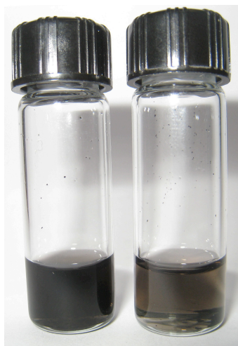
Figure S1. Experimental result of cleaving the pyrene polymer in solution. On the left, the control sample prepared with no DTT showed no change in solubility after centrifugation. On the right, the DTT-reacted sample shows a drastic change in solubility of the CNTs as a result of polymer cleavage.
