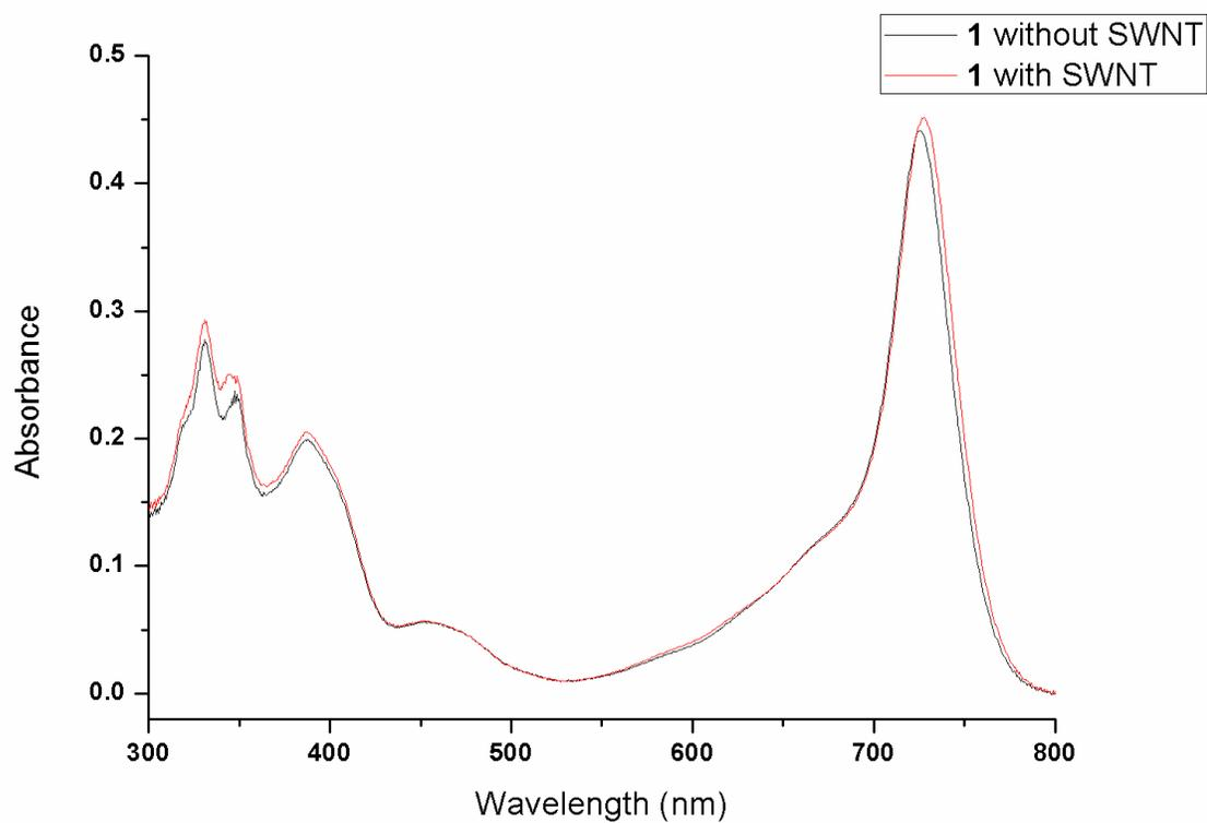
**Figure S1.** Absorbance of compound **1** in ethanol-PBS mixture (50/50, v/v). Red line: compound **1** before adsorption on to SWNT; dashed line: compound **1** after adsorption on to SWNT.
