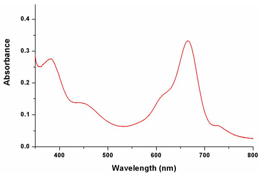
**Figure S3.** Absorbance spectrum of SWNT-adsorbed compound **1** in isopropanol. Absorption maxima in this solvent is at 666 nm.
