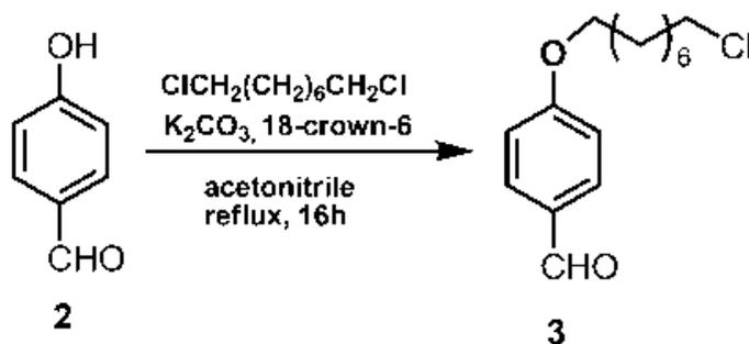
1,4-hydroxybenzaldehyde (1.25 g, 10 mmol) and 1,8 dichlorooctane (2.75 g, 15 mmol) were dissolved in acetonitrile (100 ml).  $\text{K}_2\text{CO}_3$  (2.76 g, 20 mmol) and a few crystals of 18-crown-6 were added. The reaction mixture was refluxed for 16h. Then, acetonitrile was evaporated in vacuo and extracted with water and chloroform. Organic layer as dried with  $\text{Na}_2\text{SO}_4$  and evaporated in vacuo.
