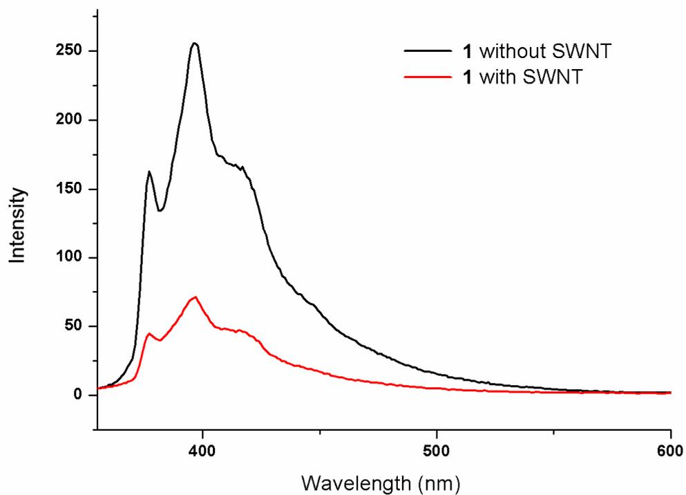
**Figure S2.** Fluorescence spectrum of compound **1** in ethanol-PBS mixture (50/50, v/v) excited at 343 nm. Red line: compound **1** before adsorption on SWNT; blue line: compound **1** after adsorption on SWNT. With equal absorbance (see Figure S1), emission of pyrene moiety of adsorbed photosensitizer was quenched three folds compared to unadsorbed one.
