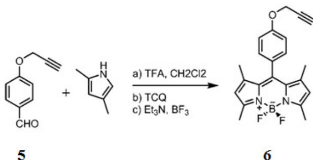
$CH_2Cl_2$  (300 ml) was purged with Ar for 30 min. 4-(prop-2-ynoxy)benzaldehyde **5** (1 g, 6.2 mmol) and 2,4-dimethyl pyrrole (1.2 g, 12.6 mmol) were added. The color of the solution turned into red after the addition of 3 drops of trifluoroacetic acid. The reaction mixture was stirred at room
