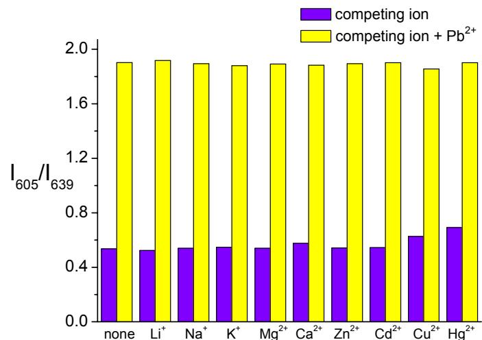
**Figure S3.** Competition experiments showing ratiometric phosphorescent response and selectivity of **1** for  $\text{Pb}^{2+}$  ions. The  $\text{Pb}^{2+}$  (1 equiv.) was added after solutions of **1** in  $\text{CH}_3\text{CN}$  ( $3.5 \times 10^{-5}$  mol/L) had been incubated with 1 equivalent of metal ions. ( $\lambda_{\text{ex}} 501$  nm)
