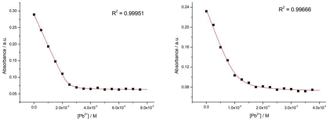
**Figure S13.** Absorbance at 534 nm as a function of Pb<sup>2+</sup> concentration and its theoretical fit for the 1:1 binding of complex **1** (left) and **2** (right) with Pb<sup>2+</sup> in CH<sub>3</sub>CN/CH<sub>2</sub>Cl<sub>2</sub> (1/1); the log *K* was calculated to be 6.63 ± 0.06 and 6.20 ± 0.15 respectively, indicating weaker binding by **2**.
