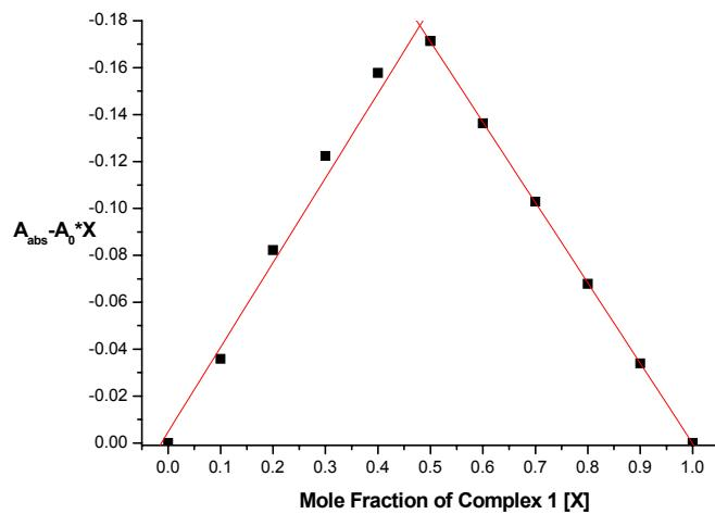
**Figure S4.** Job's plot of UV-vis data for  $\text{Pb}^{2+}$  binding by **1** in  $\text{CH}_3\text{CN}$  (concentration =  $5.3 \times 10^{-5}$  M), indicating 1:1 binding.
