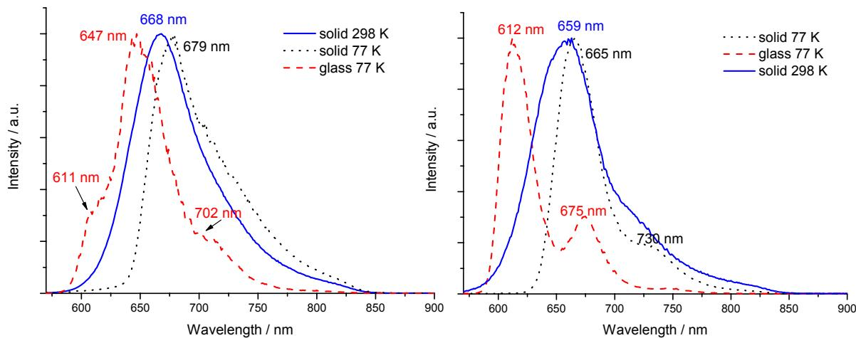
**Figure S1.** Left: Normalized emission spectra of **1** (left;  $6.8 \times 10^{-5} \text{ mol/L}$ ) and **2** (right;  $4.2 \times 10^{-5} \text{ mol/L}$ ) in solid state and 77 K glass.
