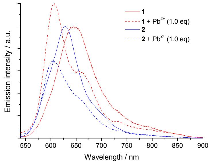
**Figure S9.** Emission spectra of **1** and **2** (normalized,  $2 \times 10^{-5}$  M,  $\lambda_{\text{ex}}$  501 nm) in CH<sub>3</sub>CN/CH<sub>2</sub>Cl<sub>2</sub> (1/1), and relative changes upon addition of Pb<sup>2+</sup> (1 equiv.).
