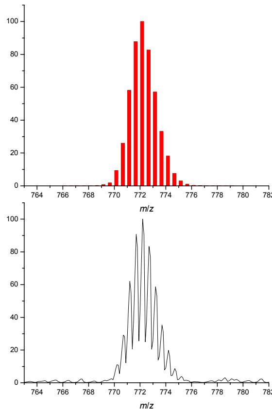
**Figure S6.** ESI-MS for 1:1  $[1 + \text{Pb}]^{2+}$  species ( $m/z = 772.2$ ) using declustering potential of 50 V in  $\text{CH}_3\text{CN}$  (top: calculated isotopic distribution with 0.5 amu separation between peaks). N.B. Cooperative 2:2 binding, which would afford 0.25 amu separations, can be disregarded (additional evidence: non-sigmoidal binding curve gives excellent fit for 1:1 binding; Hill plot does not show positive cooperation).
