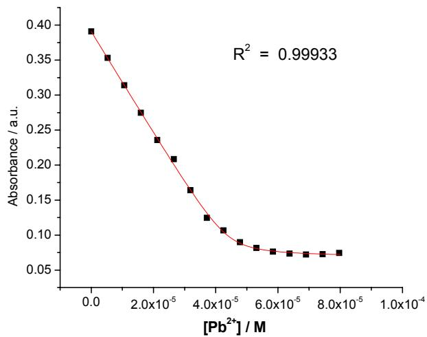
**Figure S5.** Absorbance at 534 nm as a function of  $\text{Pb}^{2+}$  concentration and its theoretical fit for the 1:1 binding of complex **1** with  $\text{Pb}^{2+}$ .<sup>6</sup> The log  $K$  was calculated to be  $6.4 \pm 0.1$  in  $\text{CH}_3\text{CN}$ .
