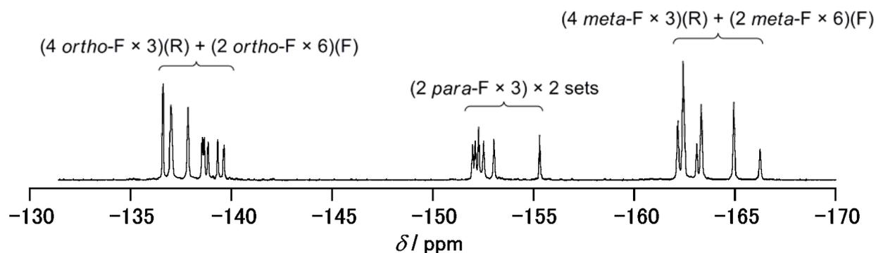
**Figure S3.**  $^{19}\text{F}$ -NMR spectrum of **3** in  $\text{CD}_2\text{Cl}_2$  at  $-60\text{ }^\circ\text{C}$ . The signals due to the rectangular conformation and figure-eight conformation are designated as (R) and (F), respectively.
