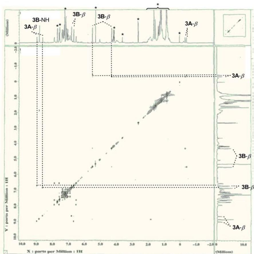
**Figure S4.**  $^1\text{H}$ - $^1\text{H}$  NOESY NMR spectrum of **3** in  $\text{CDCl}_3$  at  $-60\text{ }^\circ\text{C}$ . Correlation between the signals due to  $\beta$ -protons of **3A** and those of **3B** were observed, indicating that the conformational exchange between **3A** and **3B** is slow enough to see two separate sets of resonances but still exist at  $-60\text{ }^\circ\text{C}$ .
