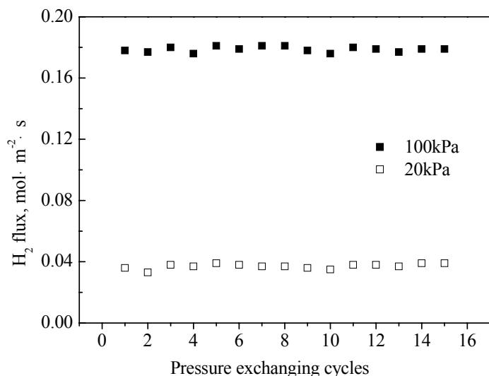
Fig.4 H<sub>2</sub> flux of as-prepared Pd-silicalite-1 membrane after successive pressure exchanging cycles between pressure difference of 100kPa and 20kPa at the operating temperature of 773K.
