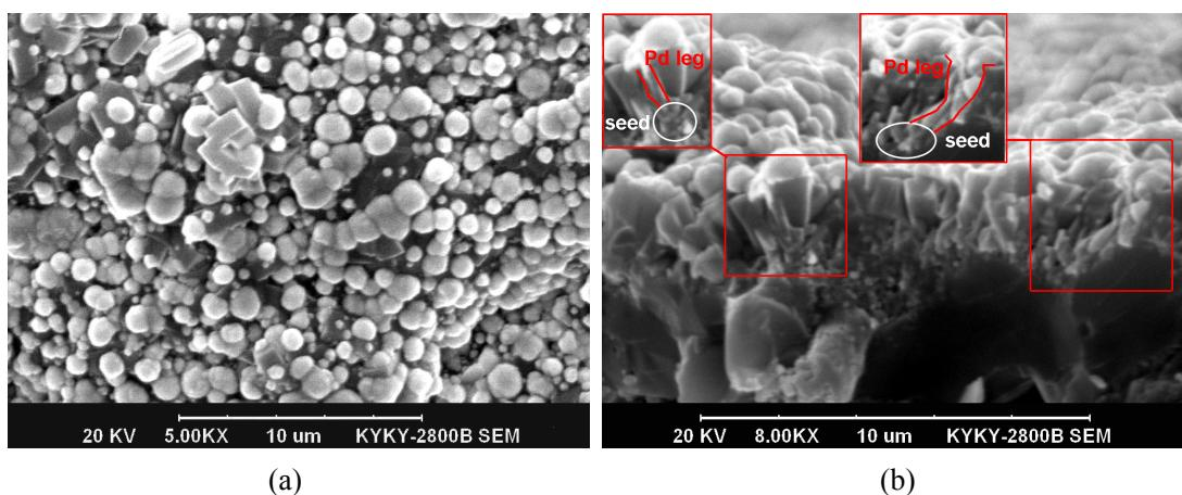
Fig.1 Pd deposits on the modified support at initial plating stage (10min): (a) surface and (b) cross section of Pd deposit on Sil-1 layer.
