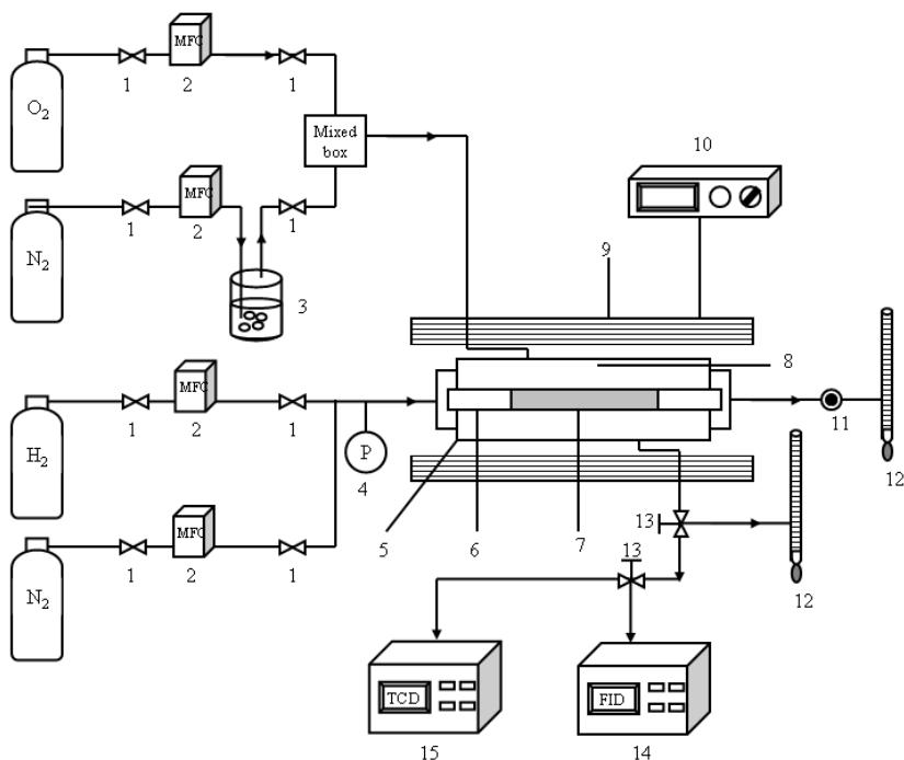
Fig.9 Apparatus used for hydroxylation of benzene
