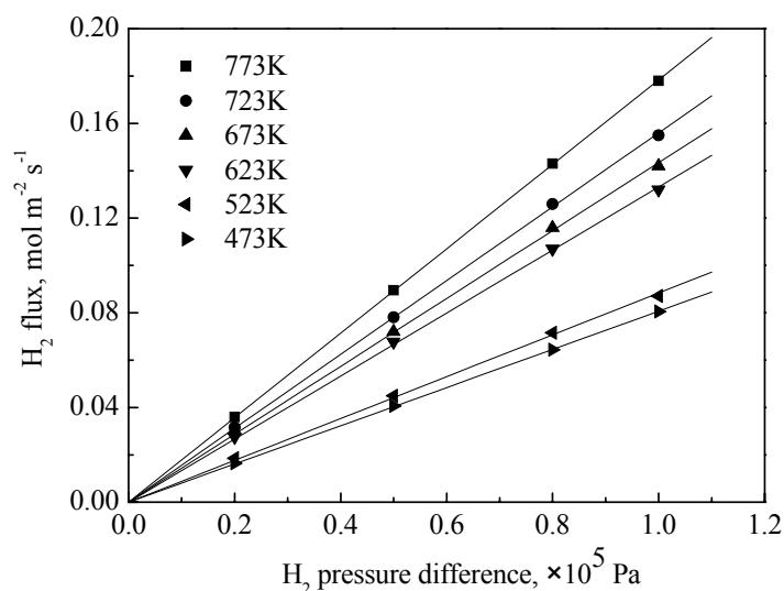
Fig.8 H<sub>2</sub> flux as a function of pressure difference at different temperatures
