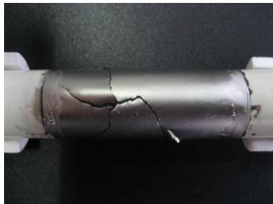
Fig. 7 Pd/Sil-1/alumina membrane after direct hydroxylation of benzene
