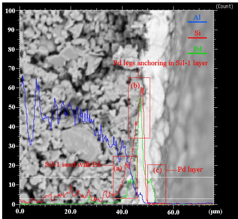
Fig.3 EPMA profiling of the Pd-silicalite-1 membrane: lining analysis
