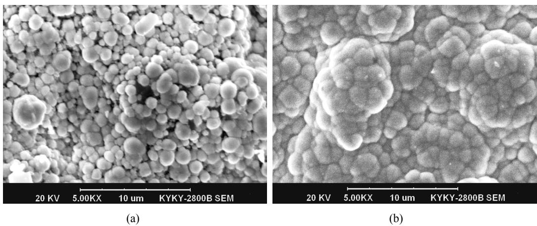
Fig.2 Pd deposits on the surface of the modified support with different deposition time: (a) 30min; (b) 60min.
