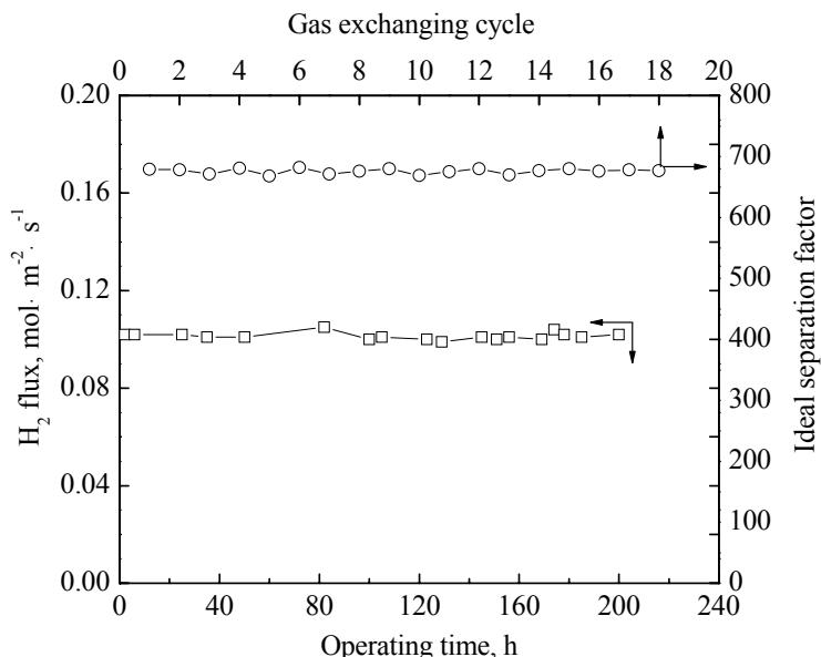
Fig.5 The stability of the Pd-silicalite-1 membrane for long term test with H<sub>2</sub> and N<sub>2</sub>.
