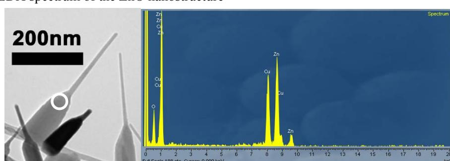
Spectrum 1, the EDX result was got from the nanoneedle section, the ration of O to Zn is 1.1.
