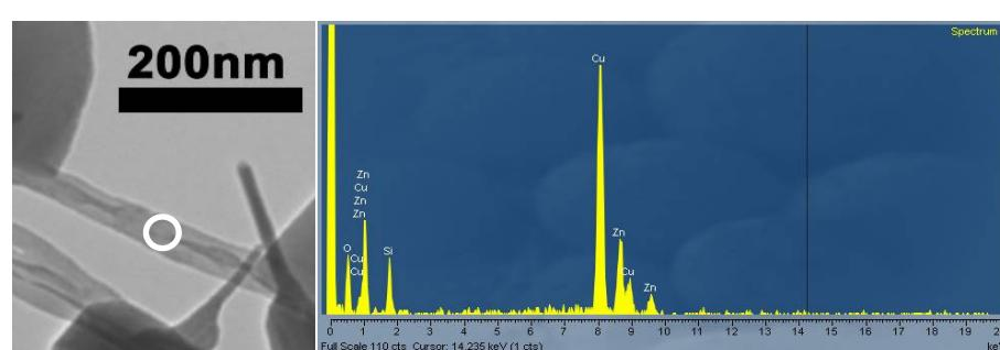
Spectrum 2, the EDX result was got from long nanowires on which the ZnO needles standing, the ratio of O:Si:Zn≈3:1:1.
