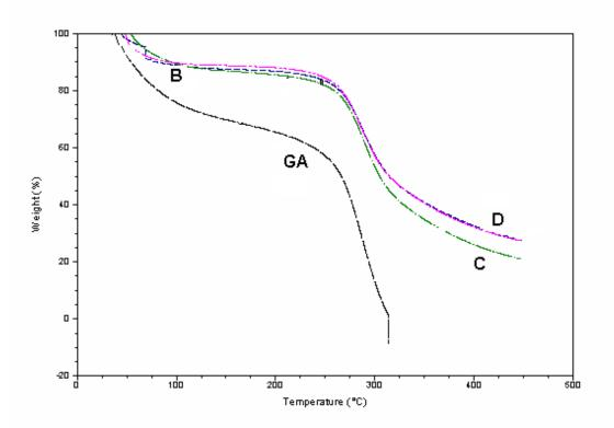
Thermogravimetric Analyser (TGA) studies were carried out to study the effect of thermal stability of collagen samples crosslinked with GA and other ionic liquids. The results show that collagen samples crosslinked with ionic liquids exhibit higher thermal stability compared to GA crosslinked sample. This shows better crosslinking efficiency (as evidenced by IR results suggesting strong coordinate / H-bonding interactions of the amide nitrogen) of the ionic liquids over GA crosslinked sample.
