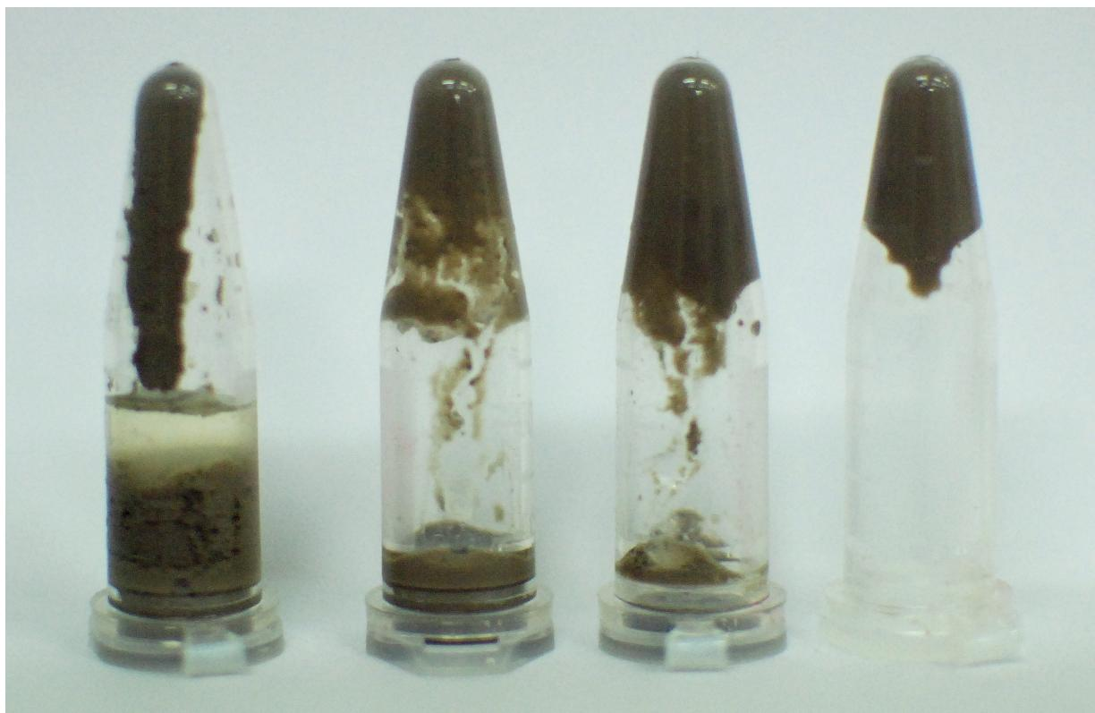
A suspension of 2 wt%, 5wt%, 7wt%, and 10wt% of ND-**1** (from left) in [bmim][PF<sub>6</sub>] was mixed in an agate mortar with a pestle for 5 min, and centrifuged at 1200 rpm for 1 min.
