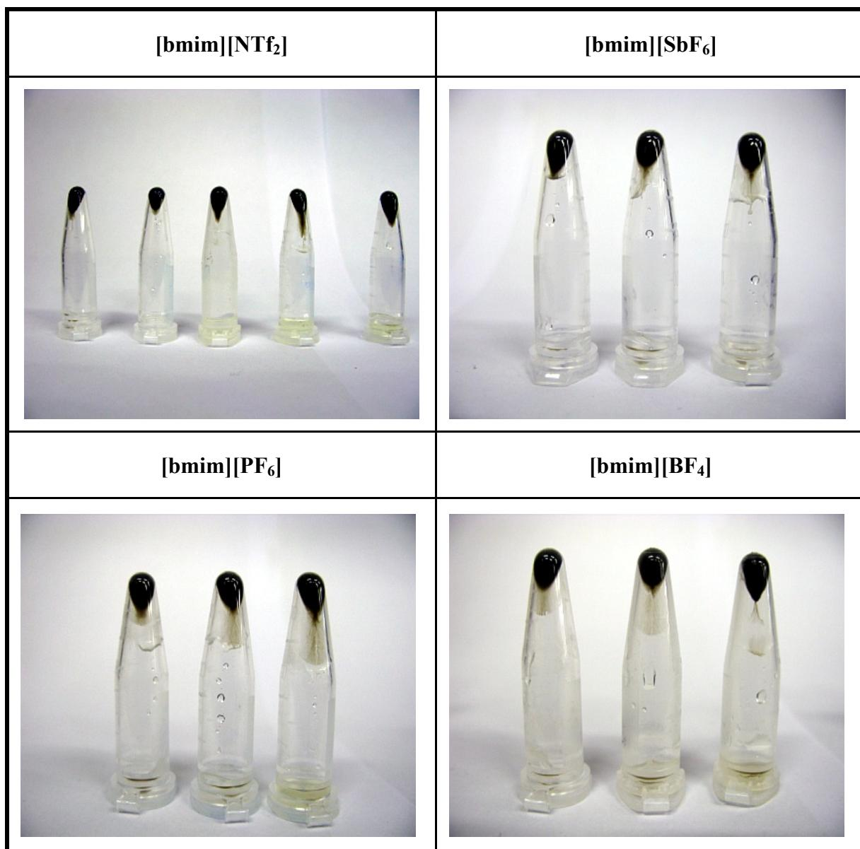
A suspension of ND-**1** (5 mg) in [bmim][NTf<sub>2</sub>] (100 mg, 200 mg, 300 mg, 400 mg, and 500 mg, from left to right) was mixed in an agate mortar with a pestle for 15 min, and centrifuged at 13000 rpm for 3 h. For other ionic liquids, 100mg, 200 mg, and 300 mg of ionic liquid was used (from left to right).
