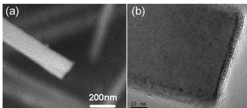
**Fig. S2** SEM (a) and TEM (b) images showing BN-coated flat nanowire tips. The nanowires are entirely sealed with BN layers that effectively prevent their decomposition.
