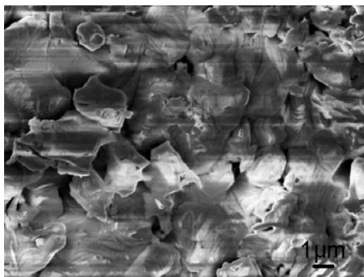
**Fig. S3** SEM image of an uncoated bulk CaS:Eu crystal fabricated without use of boron oxide.
