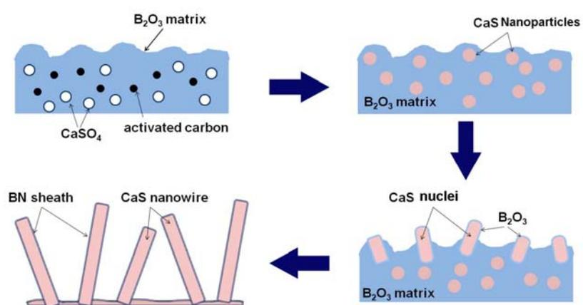
**Fig. S4** Schematic illustration of the nanowire growth mechanism.
