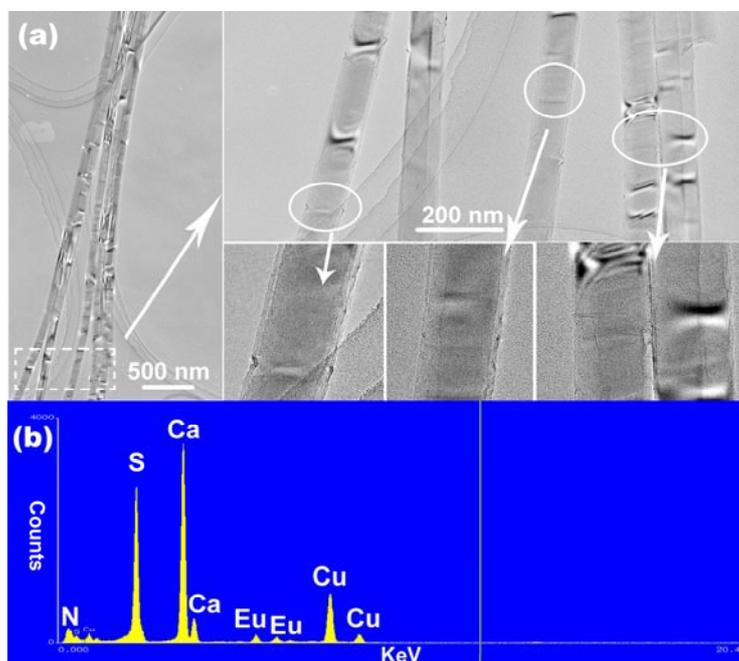
**Fig. S1** (a) TEM images of several nanowires, showing that all of them are sheathed with BN layers. (b) A typical EDS spectrum taken from the individual nanowire in (a).
