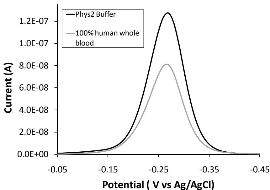
**Fig. S15** E-DNA sensor response to human whole blood. A ~37% signal reduction is evident when the sensor was transferred from a Phys2 buffer to the whole blood matrix. The reduction in current is probably due to the differences in the viscosity and ionic strength, which is known to affect the MB current in E-DNA sensors.
