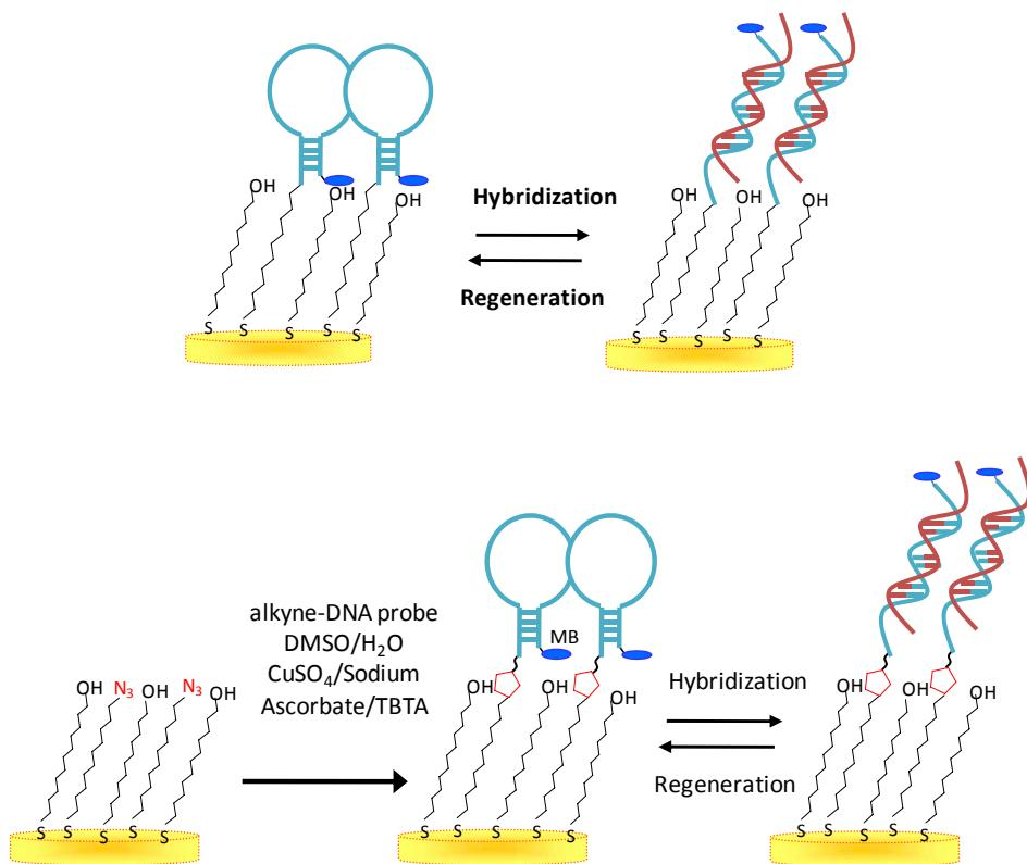
**Fig. SI3** The conventional (top) and “click” chemistry-based (bottom) E-DNA sensor constructs.
