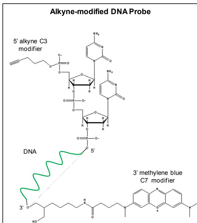
**Fig. S12** Structures of the probe DNA used in the conventional (top) and “click” chemistry-based (bottom) E-DNA sensors.
