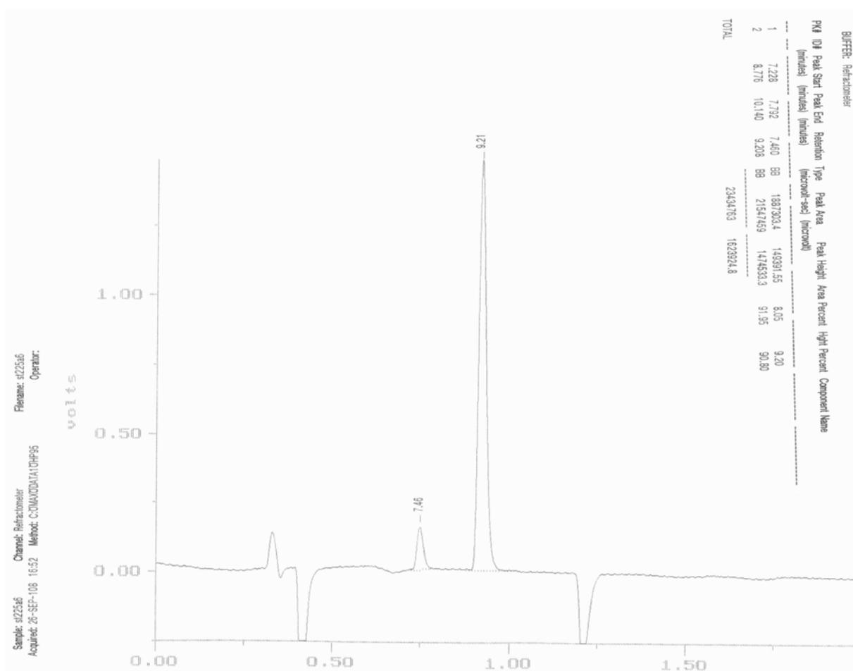
*cis*: 79% *ee*, Spectral data were consistent with literature values.<sup>4</sup> Enantiomeric ratio was determined by HPLC (AD-H, 1.0 mL / min; 1% *i*PrOH/hexane: (*R*)  $t_1 = 7.6$  min, (*S*)  $t_2 = 8.5$  min.
