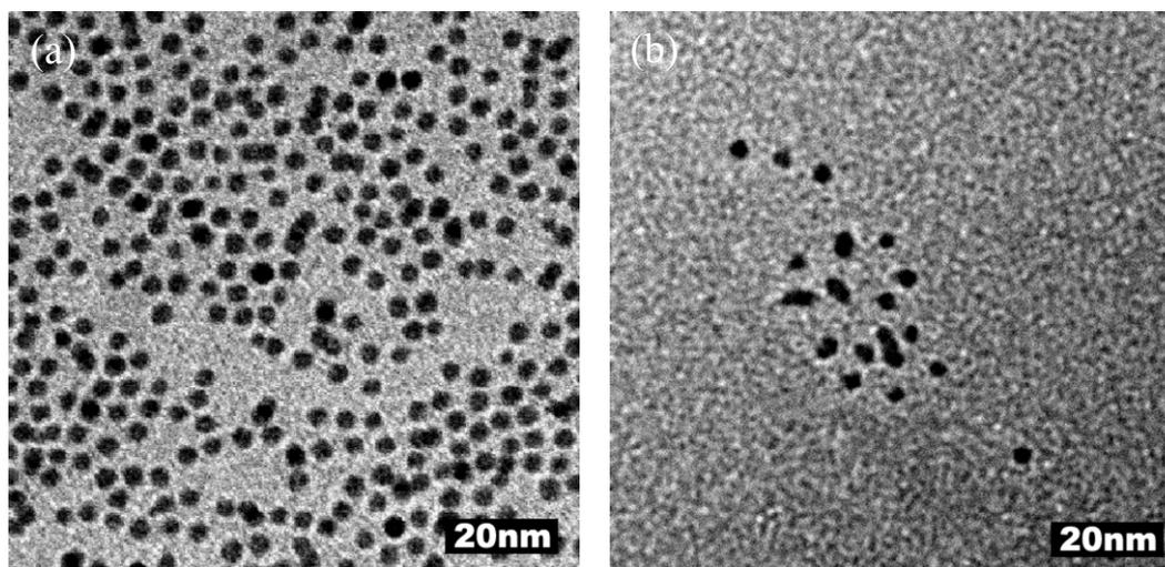
**Fig. S1** TEM images of (a) Pd NPs and (b) detection-probe conjugated Pd NPs.
