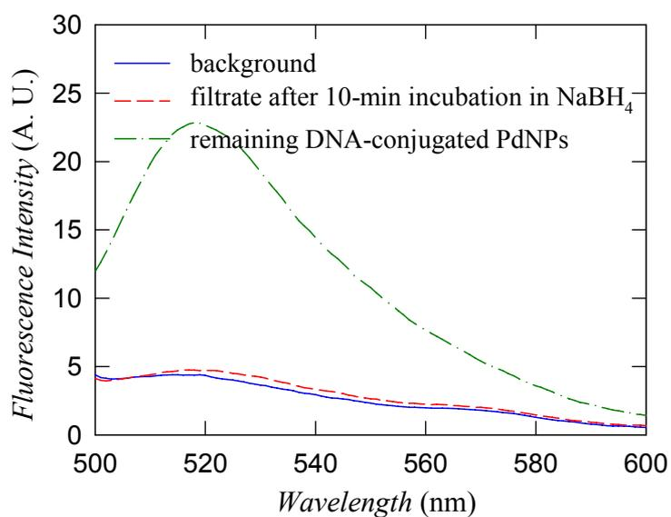
**Fig. S2** Fluorescence spectra of oligreen-containing solutions. The background corresponds to the spectrum obtained in a solution containing no DNA-conjugated Pd NPs, the filtrate after 10-min incubation in NaBH<sub>4</sub> corresponds to the spectrum obtained with the filtrate after NaBH<sub>4</sub> treatment of DNA-conjugated Pd NPs, and the remaining DNA-conjugated Au NPs corresponds to the spectrum obtained from residual DNA-conjugated Pd NPs after filtration.
