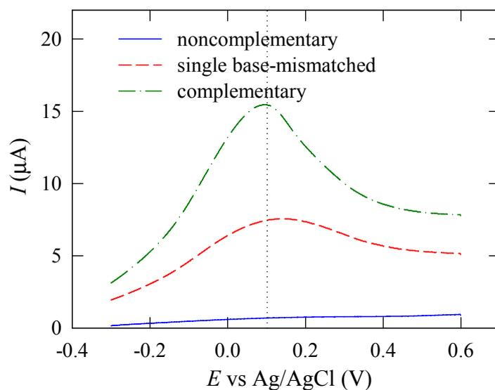
**Fig. S6** Linear sweep voltammograms obtained after 20-sec incubation in a 0.1 M borate buffer solution (pH 11) containing 5 mM NaBH<sub>4</sub> (at a scan rate of 50 mV/s) after incubation with a solution containing 1 nM complementary, single base-mismatched, or noncomplementary target DNA.
