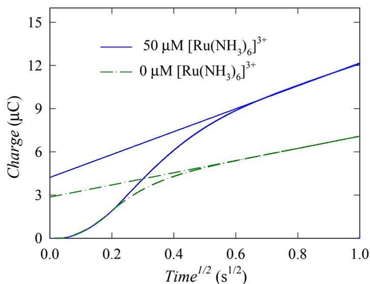
**Fig. S4** Chronocoulometric data obtained at capture probe-modified DNA-sensing electrodes in a 10 mM Tris buffer solution (pH 7.4) in the presence and absence of 50  $\mu\text{M}$  [Ru(NH<sub>3</sub>)<sub>6</sub>]<sup>3+</sup>.
