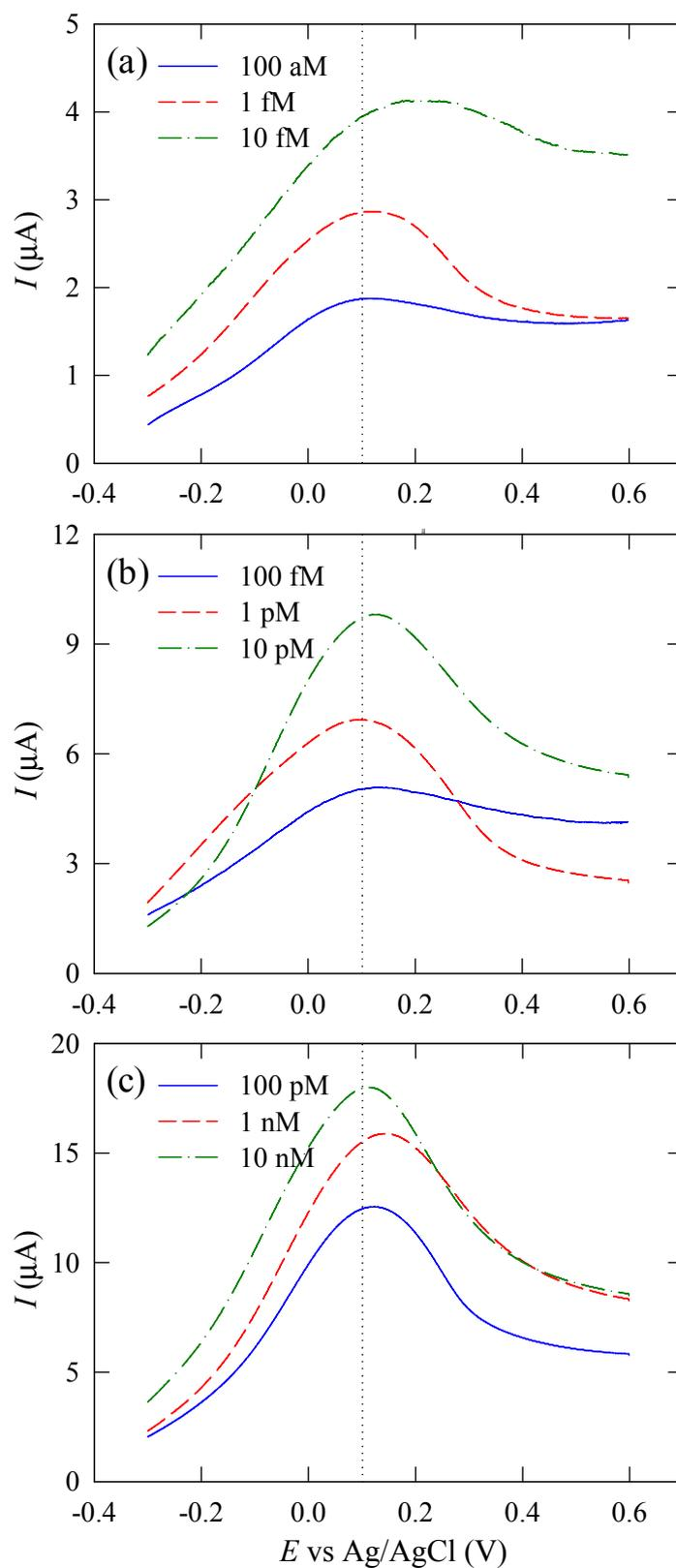
**Fig. S5** Concentration dependence of linear sweep voltammograms obtained after 20-sec incubation in a 0.1 M borate buffer solution (pH 11) containing 5 mM  $\text{NaBH}_4$  (at a scan rate of 50 mV/s).
