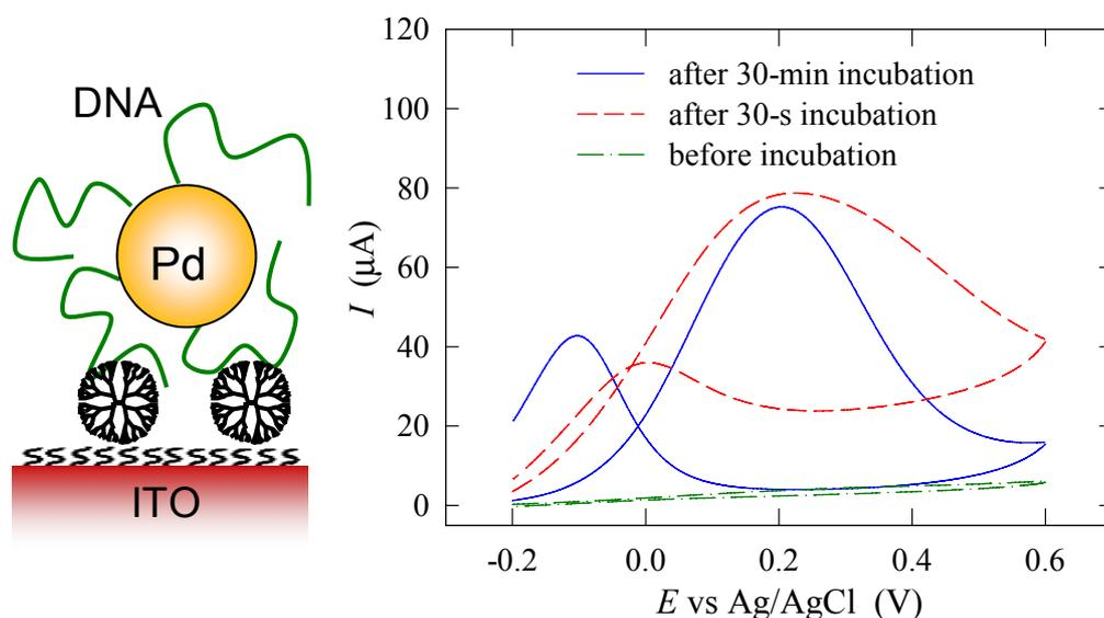
**Fig. S3** Cyclic voltammograms obtained in a phosphate buffer solution (pH 8.0) containing 2 mM hydrazine (at a scan rate of 50 mV/s) at the ITO/dendrimer electrodes on which detection probe-conjugated Pd NPs were electrostatically adsorbed, before and after incubation in a Tris buffer containing 10 mM NaBH<sub>4</sub> (pH 9).
