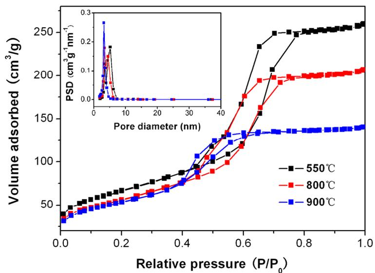
**Figure. S5** Nitrogen adsorption-desorption isotherms and the pore-size distributions of the mesoporous Ni-containing (12 mol%) alumina monoliths calcined at various temperatures.
