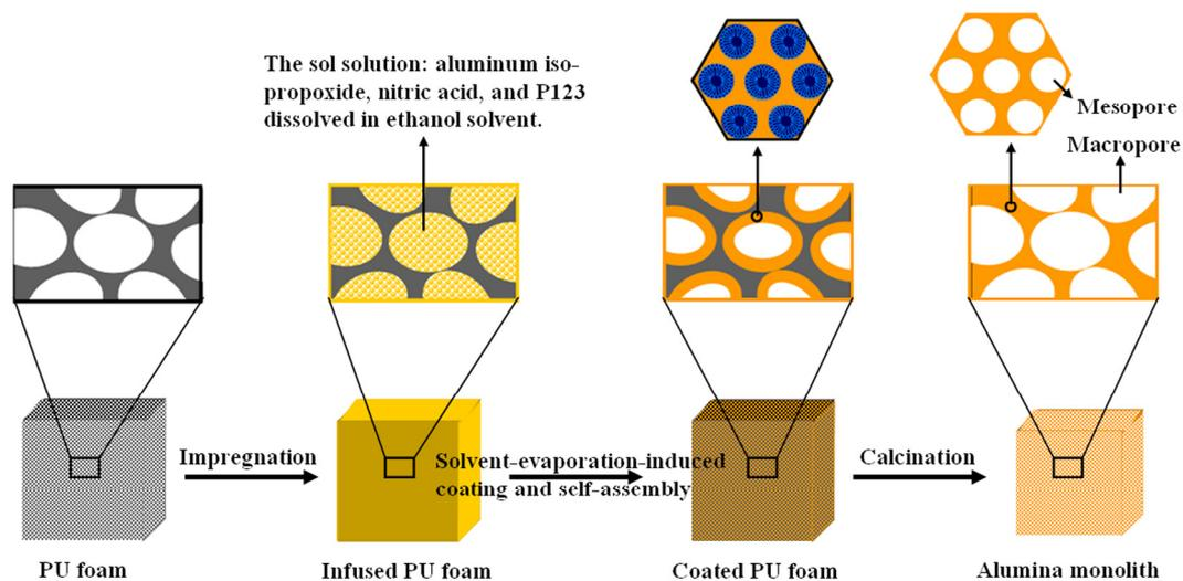
**Figure S1.** Illustration of the synthesis procedure of hierarchical porous Al<sub>2</sub>O<sub>3</sub> monoliths by using nonionic triblock copolymer and polyurethane (PU) foam as cotemplates via a solvent-evaporation-induced coating and self-assembly method.
