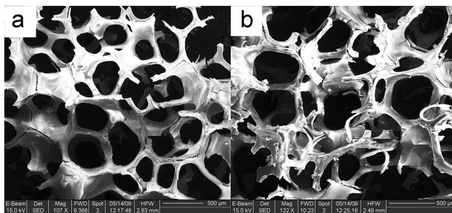
**Figure S4.** SEM images of the Ni-containing alumina monoliths (12 mol% of Ni) calcined at (a) 550 °C and (b) 900 °C.
