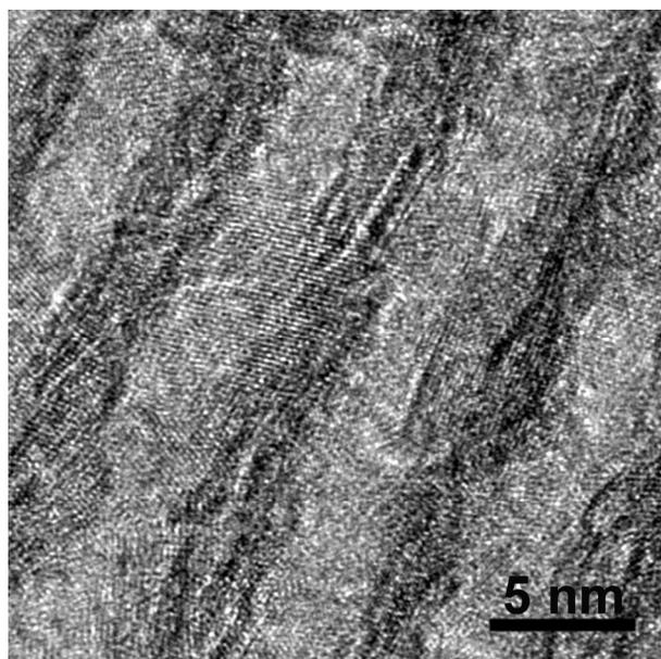
**Figure S2.** HRTEM image of alumina monolith calcined at 900 °C.
