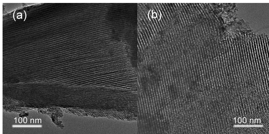
**Figure S3.** TEM images of the Ni-containing alumina monoliths (12 mol% of Ni) calcined at (a) 550 °C and (b) 900 °C.
