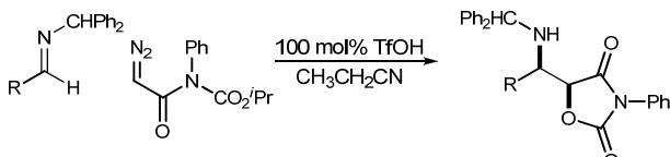
**General procedure for the *syn*-Glycolate Mannich reaction.** To a cold (-78 °C) solution of imine (1.0 equiv) and α-diazo imide (1.2 equiv) in propionitrile (1.0 mL) was added dry TfOH (1.0 equiv), and the solution was stirred at -78 °C. The reaction was quenched with satd aq NaHCO<sub>3</sub> and extracted with ethyl acetate. The organic layers were dried, concentrated, and the resulting solid was purified by silica gel flash chromatography.
