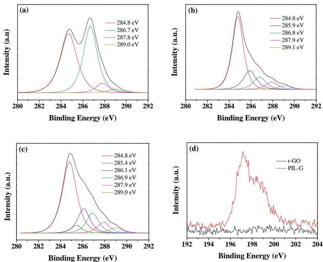
Figure S4. The XPS C 1s spectra of (a) graphite oxide (GO), (b) reduced graphite oxide (r-GO), and (c) PIL stabilized graphene sheets (PIL-G). (d) The XPS Cl 2p spectra of r-GO and PIL-G.
