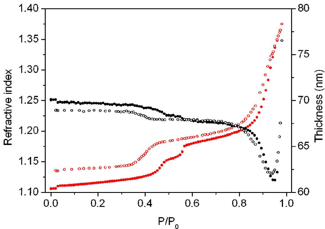
**Fig. S8** Evolution of refractive index (red) and thickness (black) of one-layer of MIL-101(Cr) film as a function of relative humidity, during water adsorption (filled circles)—desorption (open circles) cycle.
