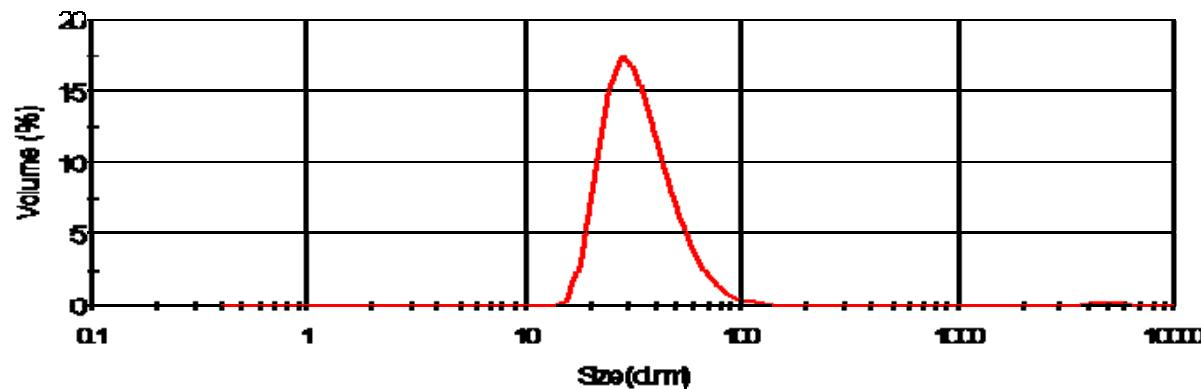
**Fig. S1** Diffusion Light Scattering size distribution curve of nanoparticles of MIL101(Cr) in water at 25 °C (Z-average 49 nm, polydispersity 0.236).
