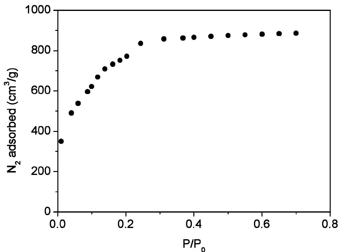
**Fig. S5** N<sub>2</sub> adsorption isotherm at 77 K in nanoparticles of MIL101(Cr) activated at 120 °C under vacuum.
