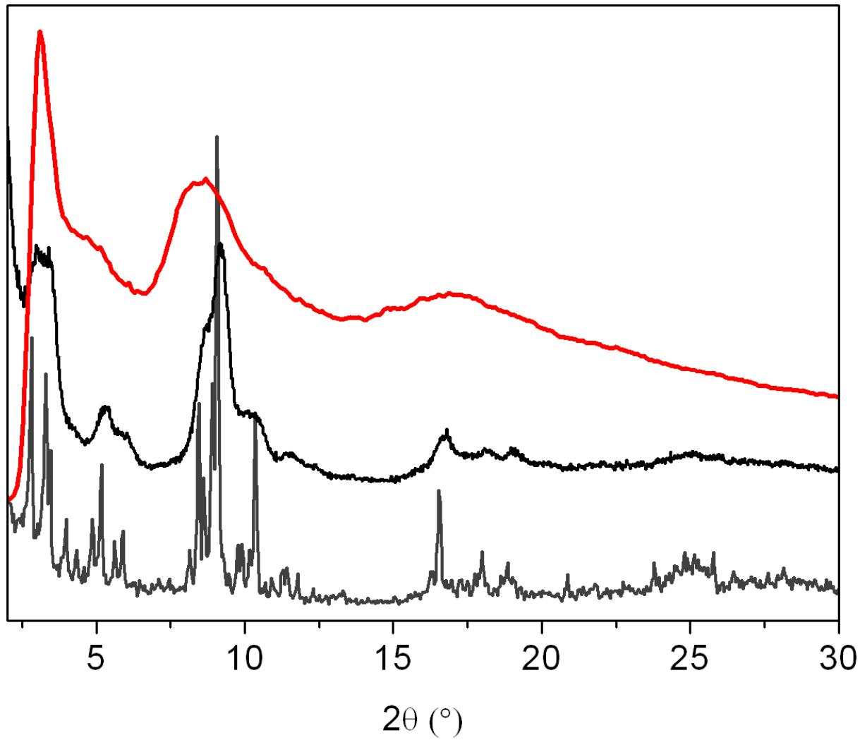
**Fig. S3** XRPD pattern of bulk (grey) and nanoparticles (black), and GI-WAXS on a thin film of MIL-101(Cr) (red).
