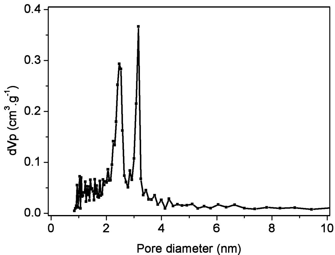
**Fig. S9** Pore size distribution plot from water adsorption study at room temperature. The plot shows the existence of two maxima centred at pore radii of ca. 2.5 nm and 3.2 nm.
