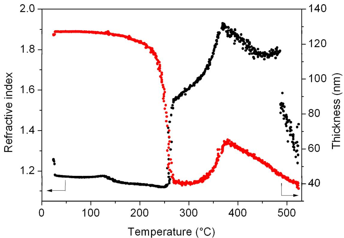
**Fig. S6** Evolutions of the refractive index (black) and the thickness (red) of one-deposition MIL-101(Cr) film upon increasing temperature. Experiment carried out at  $4\text{ }^{\circ}\text{C}.\text{min}^{-1}$  under ambient atmosphere.
