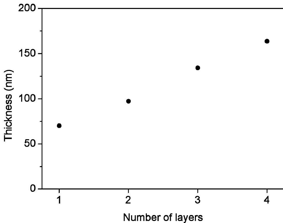
**Fig. S7** Evolution of the thickness of a thin film of MIL101(Cr) with the number of depositions by dip-coating at relative humidity null (Table 1).
