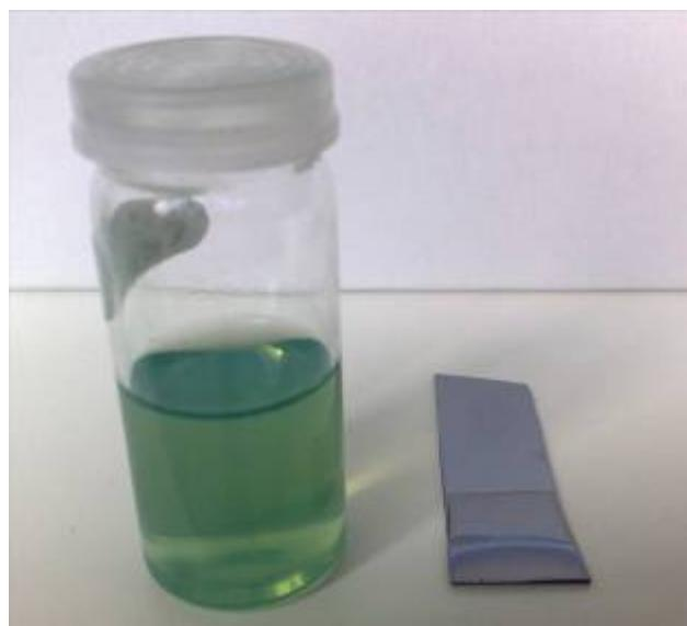
**Fig. S11** Picture of the stable suspension of MIL101(Cr) nanoparticles (left) used to dip-coat high quality optical thin films on silicon wafer(right).
