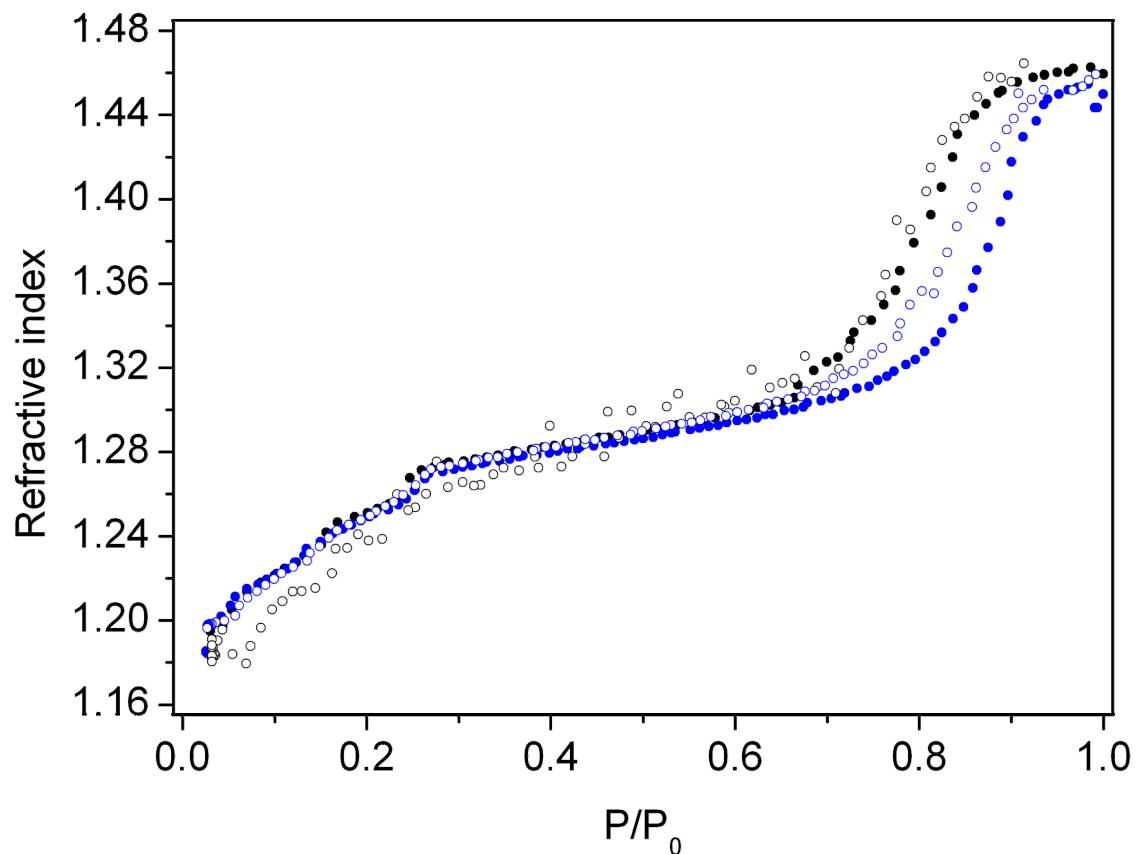
**Fig. S10** Evolution of sorbed absolute ethanol (blue) and isopropanol (black) refractive index of one-deposition of MIL-101(Cr) film upon solvent adsorption (filled) – desorption (open) cycle.
