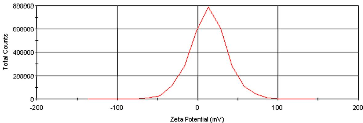
**Fig. S2** Zeta potential distribution of nanoparticles of MIL101(Cr) in absolute ethanol at 25 °C (Zeta potential 13.5 mV, conductivity 0.00484 mS/cm).
