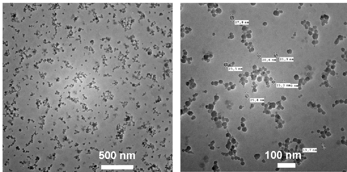
**Fig. S3** TEM images of nanoparticles of MIL101(Cr).
