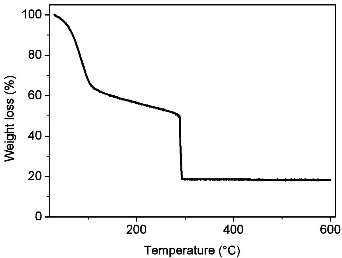
**Fig. S4** TGA curve of nanoparticles of MIL101(Cr).
