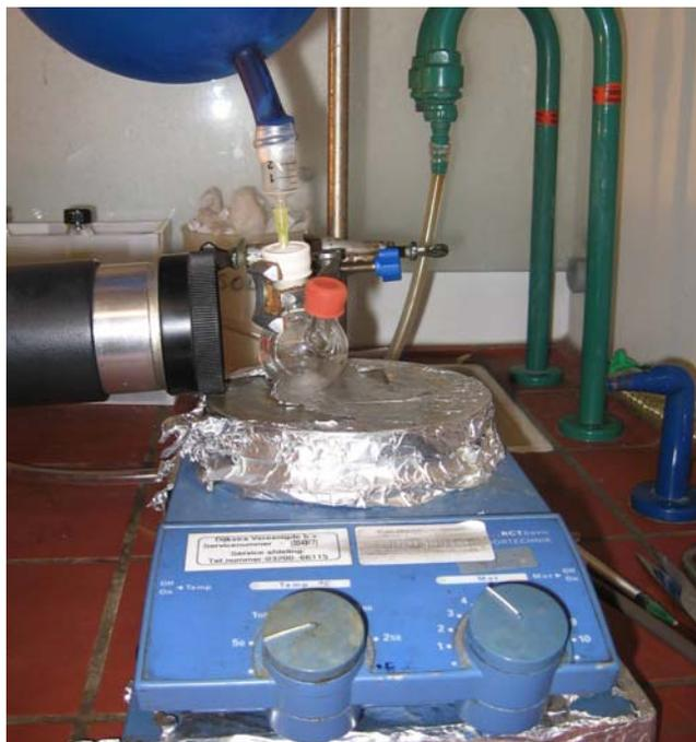
**Figure 1: Experimental setup of the photobiocatalytic oxidation/oxygenation reactions.** Instead of the projector lamp any given source for visible light can be applied. Also sunlight can be used but is not advisable in terms of reproducibility due to the varying Dutch weather conditions.<sup>1</sup>
