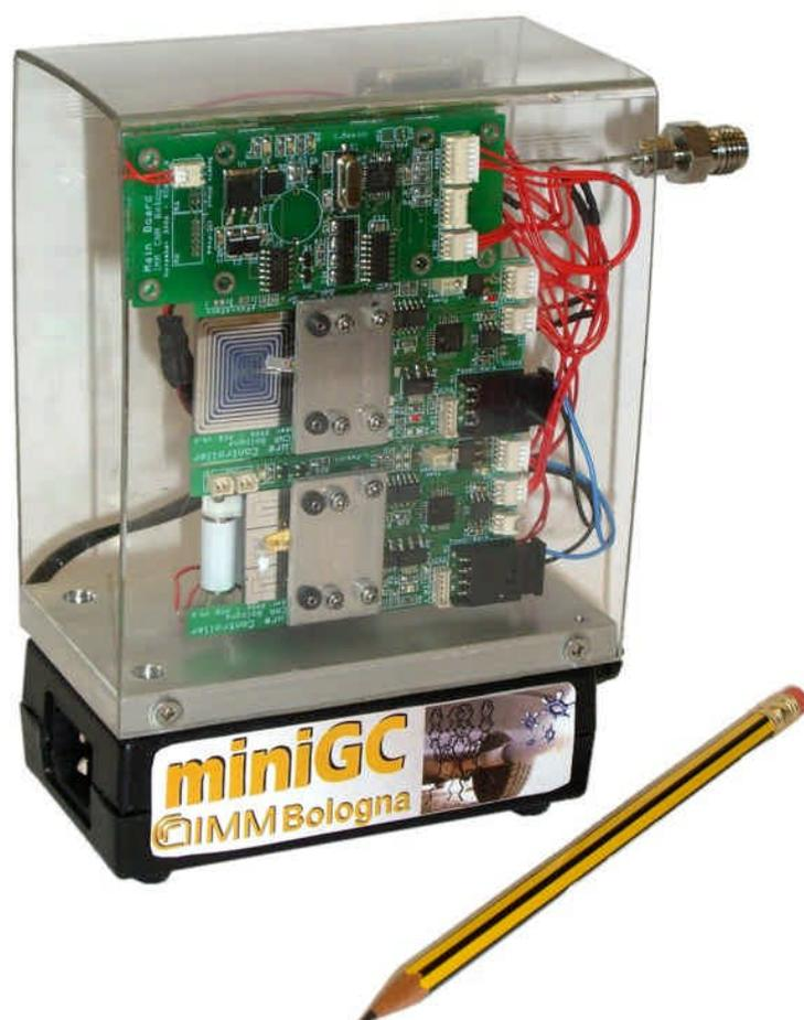
Figure S2. Prototype of the online benzene detection system.
