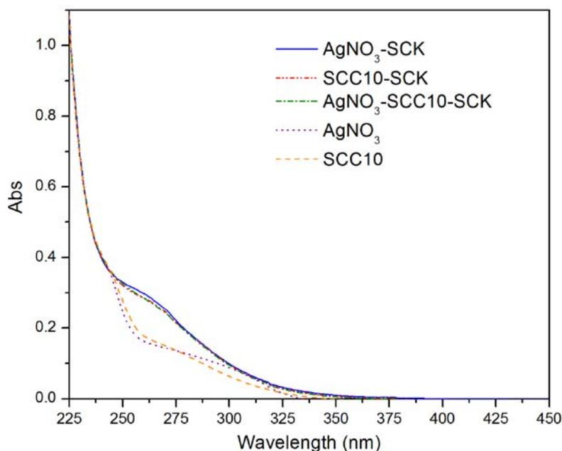
**Figure S3.** UV-vis spectra of silver-bearing nanoparticles after purification, and control samples, AgNO<sub>3</sub> and SCC10. Depletion of a UV-vis silver signal in the filtrates, following centricon centrifugal purification, combined with measurement of silver content by ICP-MS confirmed the purification of the Ag-loaded nanoparticles. The absence of any signal from 380-440 indicates the absence of large silver particles (*ca.* >10 nm).
