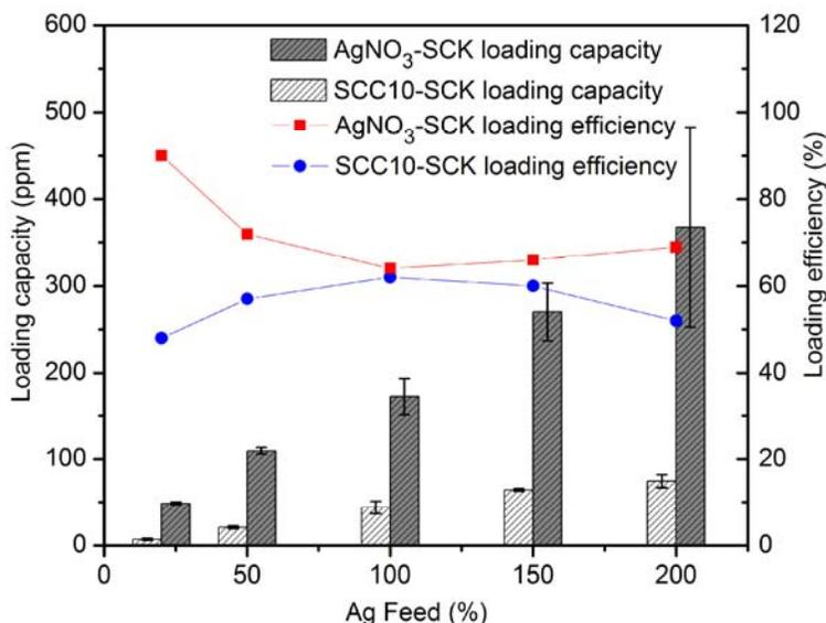
**Figure S1.** Ag loading capacities (left axis) and efficiencies (right axis) of AgNO<sub>3</sub>-SCK and SCC10-SCK with different silver feed (20%, 50%, 100%, 150%, 200% with respect to the combined total theoretical moles of acrylic acid and amide residues in the polymer for AgNO<sub>3</sub>-SCK, and with respect to the polymer weight of the SCK solution for SCC10-SCK, respectively).
