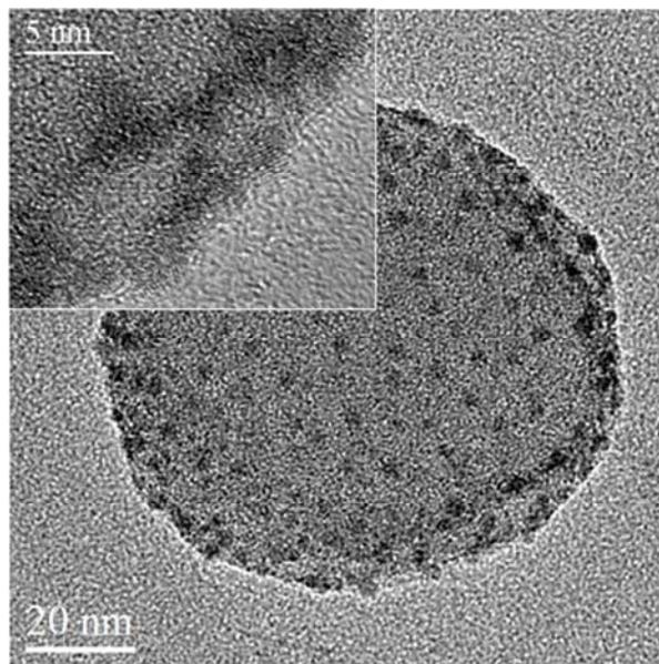
**Figure S2.** High-resolution TEM image of AgNO<sub>3</sub>-SCK nanoparticles with elemental silver on the surface, which were measured to have metallic Ag lattice spacing = 2.36 Å = d<sub>Ag(111)</sub>. (For clarity reason, a relatively larger than average nanoparticle was selected to identify the lattice spacing of the elemental silver).
