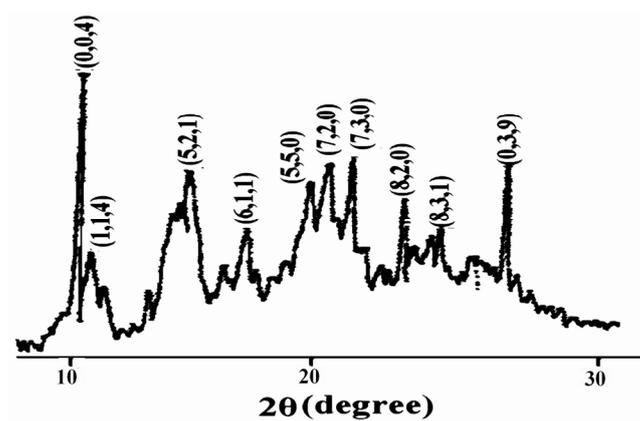
**Figure S10.** XRD pattern of compound **1** after the catalysis reaction with the indexes of some selected diffractions (the crystallographic index of the polycrystals was based on the least-square fitting of the cell parameters and the  $2\theta$  of these diffractions).
