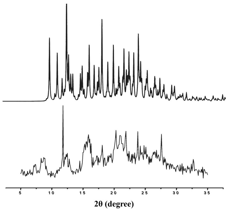
**Figure S9.** XRD pattern of compound **1** data after the reabsorb of methanol (bottom) and simulation of the XRD according to single crystal diffraction of compound **1** (top).
