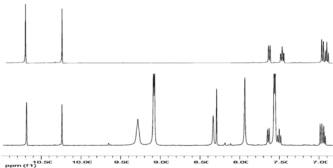
**Figure S4.**  $^1\text{H-NMR}$  spectra ( $\text{d}_6\text{-DMSO}$ ) of salicylaldehyde (top picture) and compound **1** triangle adsorbed salicylaldehyde (bottom)
