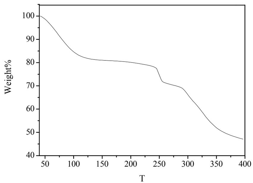
**Figure S6.** TGA curve of deslovent compound **1** immersed in methanol for 4 hours (bottom one).
