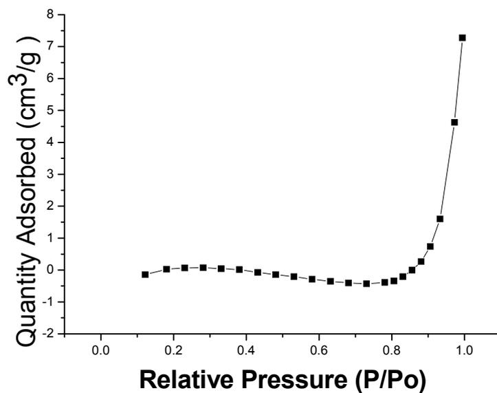
**Figure S7.** Gas adsorption isotherms for the uptake of N<sub>2</sub> (77 K) of the crystalline powder of the as-synthesized compound **1**
