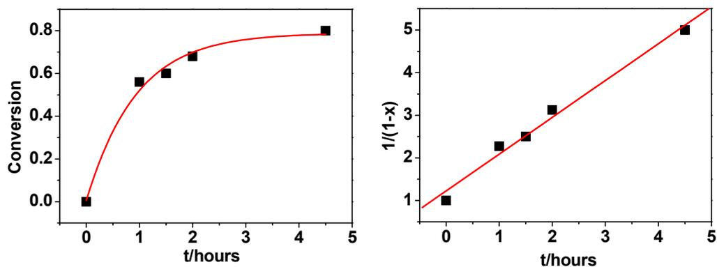
Conversion (%) vs time (left) and linear fit according to the second grade reaction, x is the conversion (right).
