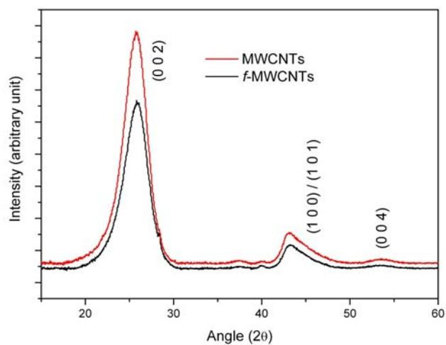
**Figure S7.** XRD spectra of pristine MWCNTs (red line) and *f*-MWCNTs (black line).
