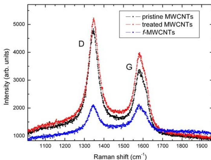
**Figure S6.** Raman spectra of pristine MWCNTs (black line) and *f*-MWCNTs (blu line) at 514.5 nm. Red line refers to a sample of MWCNTs which was treated in DMF at 160 °C for three days (standard reaction protocol) followed by the same washing/filtration/sonication/work-up procedures.
