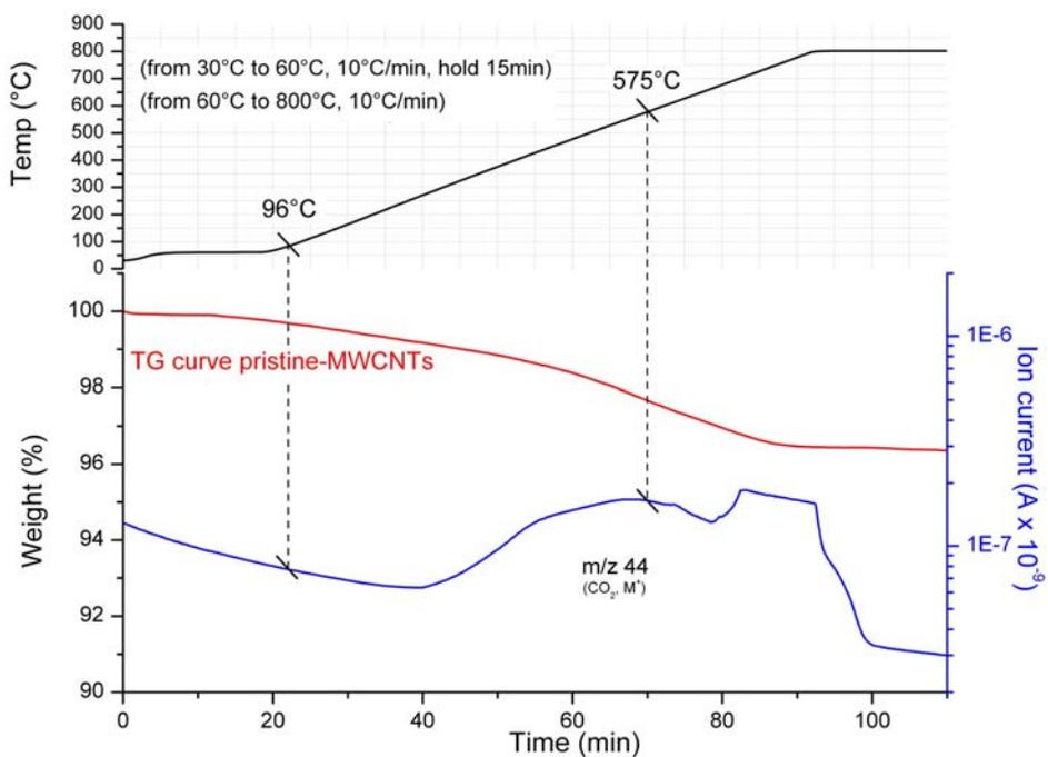
**Figure S2.** TGA-MS of pristine MWCNTs from 60 to 800 °C.  $\text{CO}_2$  ( $m/z = 44$ ) evolution have been monitored throughout the range of temperatures.
