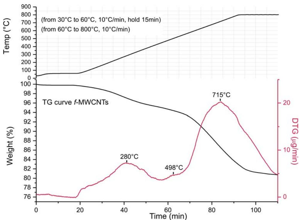
Figure S3. TGA-DTG of *f*-MWCNTs from 60 to 800 °C.
