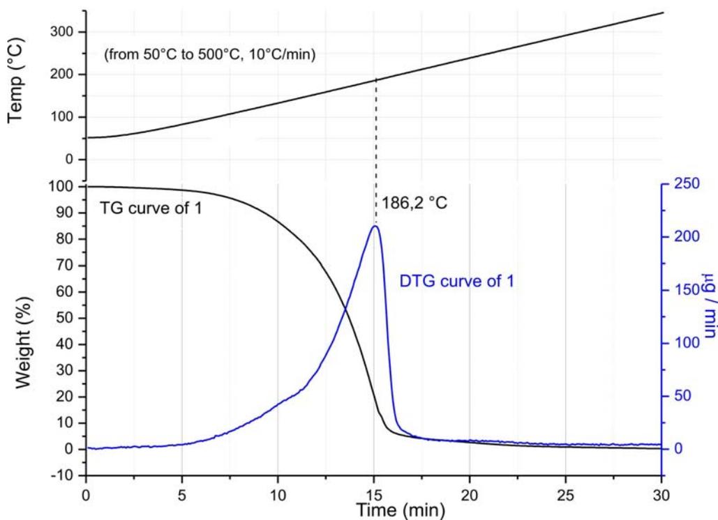
Figure S4. TGA-DTG of nitron 1 from 50 to 500 °C.
