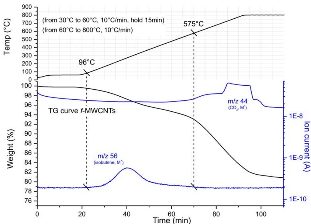
**Figure S1.** TGA-MS of *f*-MWCNTs from 60 to 800 °C. Isobutene ( $m/z = 56$ ) and  $\text{CO}_2$  ( $m/z = 44$ ) evolution have been monitored throughout the range of temperatures.
